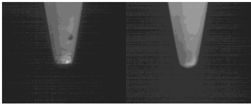
Figure 20 Heated nozzle without/with back pressure
