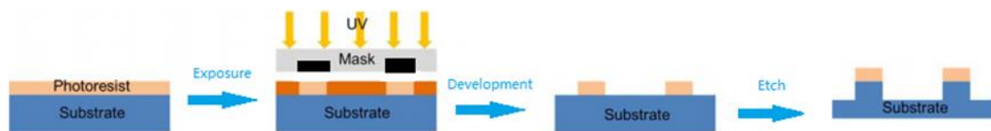
Figure 1 the process of the lithography-based microfabrication
