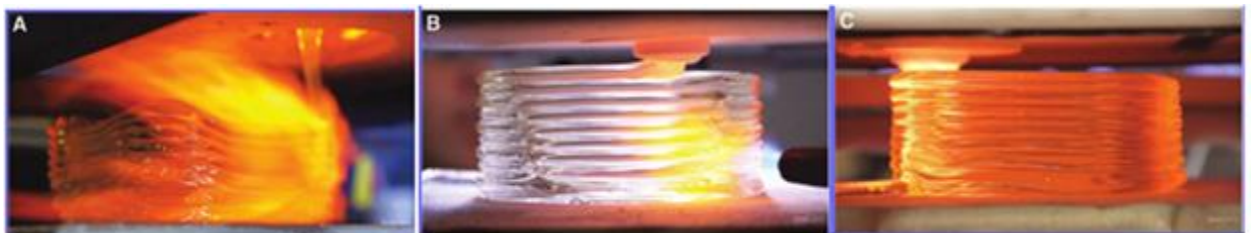
Figure 7 (A) Evolution of the printing process from its early stages (B) through the introduction of a nozzle (C) to the current setup with an annealing chamber. From [39]
