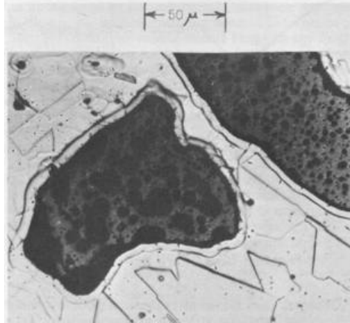
Figure 2.3. Zone of fission fragment damage in a dispersion fuel [24]
