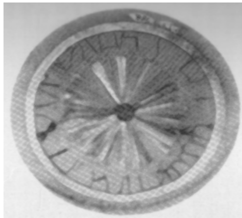
Figure 2.1. Cross-section of a solid oxide \text{UO}_2 fuel pellet [23]
