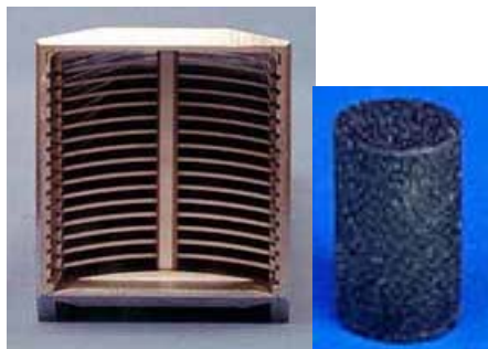
Figure 1.2. Comparison of Plate-type fuel vs. Pellet fuel
