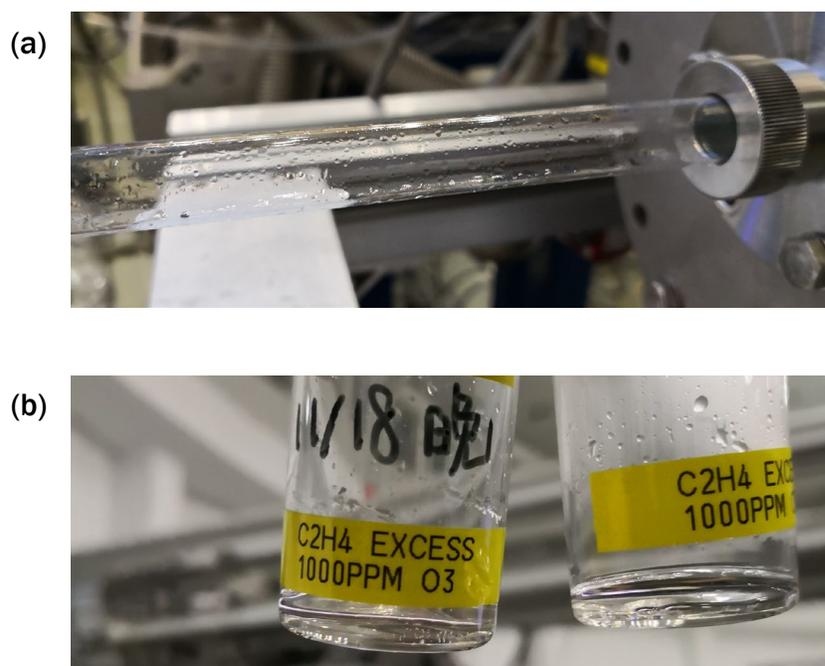
**Figure 6.6. Direct photographs of (a) highly viscous liquid accumulated on the inner wall of the flow reactor and (b) liquid sample collected with pungent odor and faint yellow color.**
