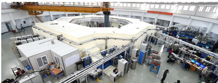
**Figure 3.22. Overview of HLS-II at NSRL, Hefei, China, with energy of 800 MeV and constant beam current 400 mA.**
