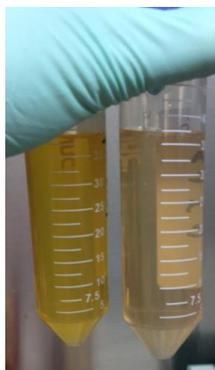
**Figure 5.7** FeCl<sub>3</sub> solutions on Day 2. Left: 0.005M FeCl<sub>3</sub> Right: 0.005M FeCl<sub>3</sub> with acetic acid
