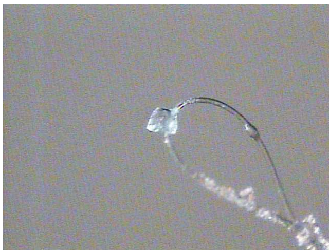
Figure 6.4 Photograph of single crystal of NiBTTB (size (mm) – 0.12 x 0.12 x 0.06)
