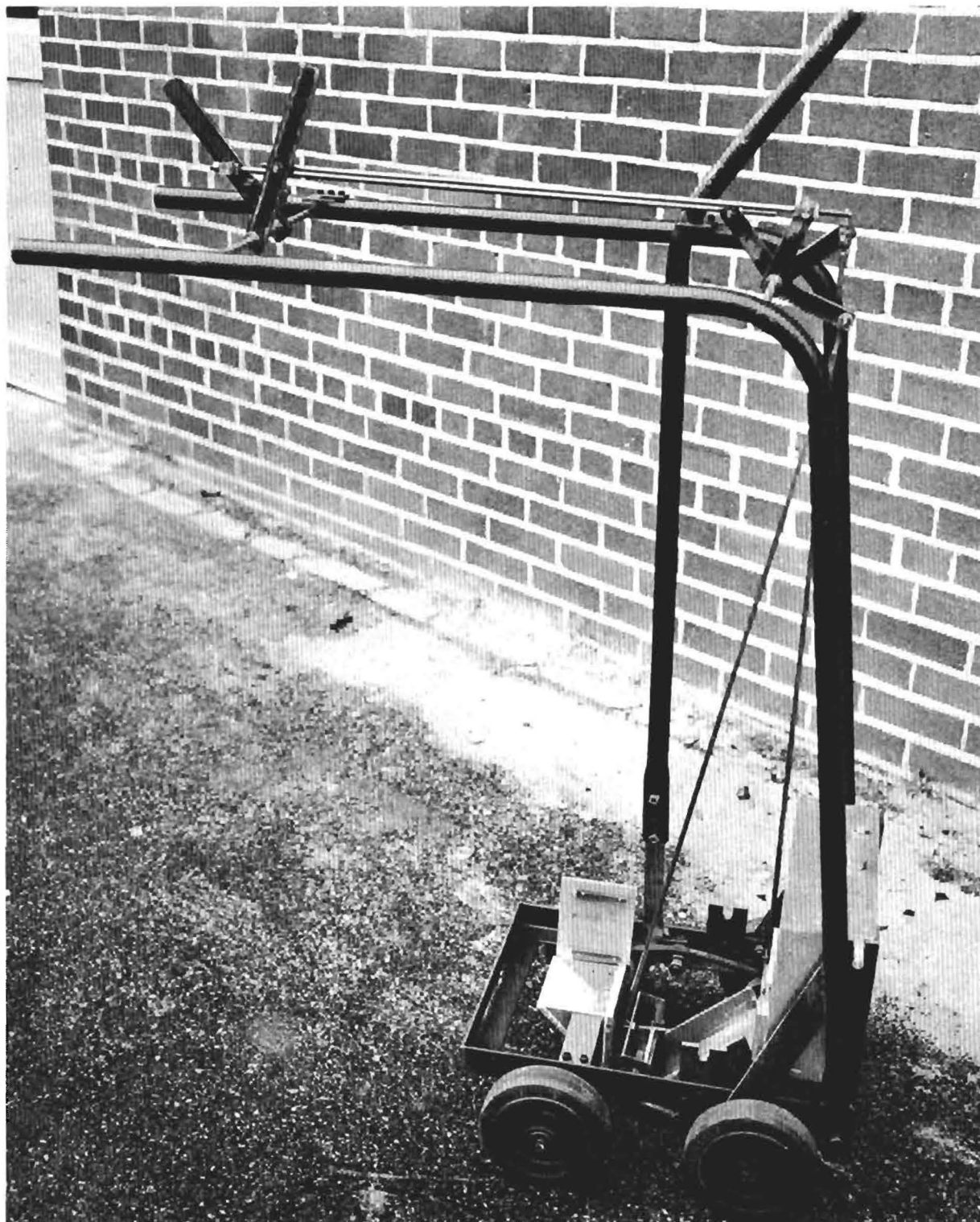
Figure 1. Experimental Hot-melt Stripe Applicator.
