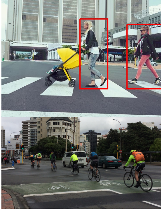
Figure 3.11: Examples where Object Detection fails to detect objects
