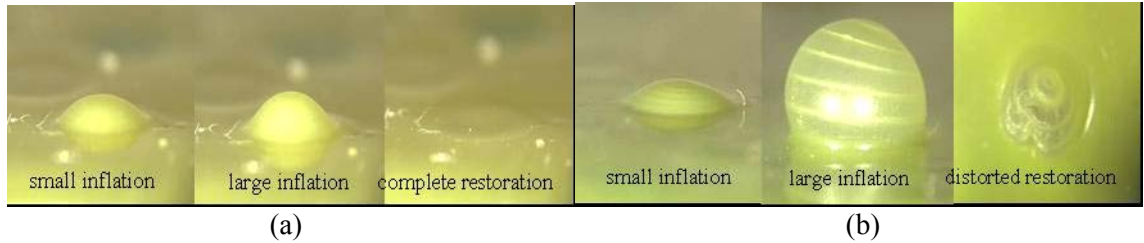
Figure 2.14. Shape comparison of (a) endoskeletal bubble and (b) pure-bubble
