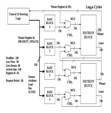
Figure 3. FPGA Hardware Architecture: Recirculating Shuffle-Exchange Network (Field Length in Bits)
