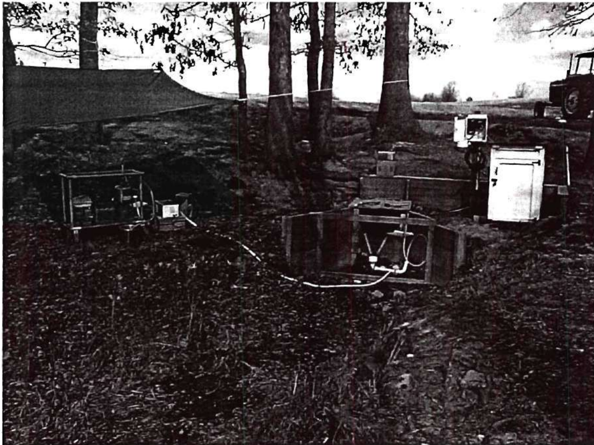
Figure 2.3 View looking east from the wetland showing monitoring and sampling instrumentation at the spring. Left to right are: flow-through centrifuge and peristaltic pump assembly, flume protected from animals, data logger, and housing for SIGMA sampler.
