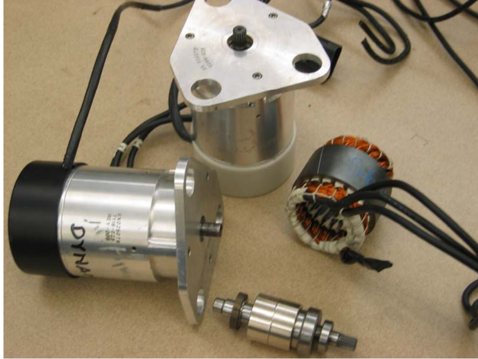
Figure 2.1: BLDC motors including a stator and a rotor.
