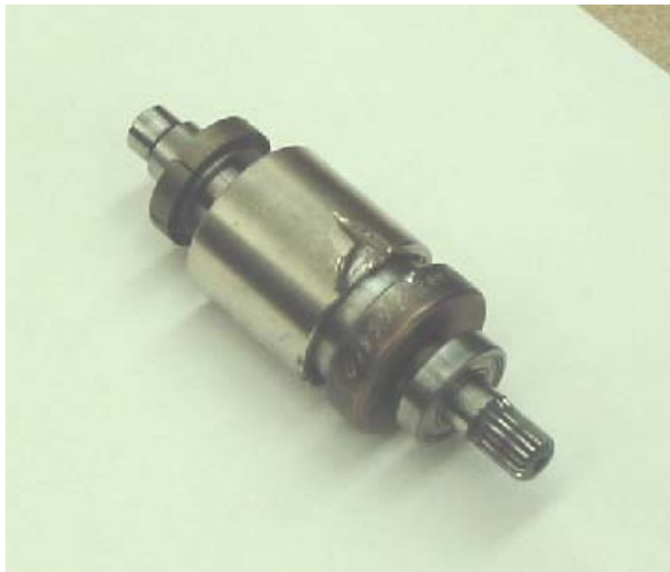
Figure 4.6: Broken magnet defect.
