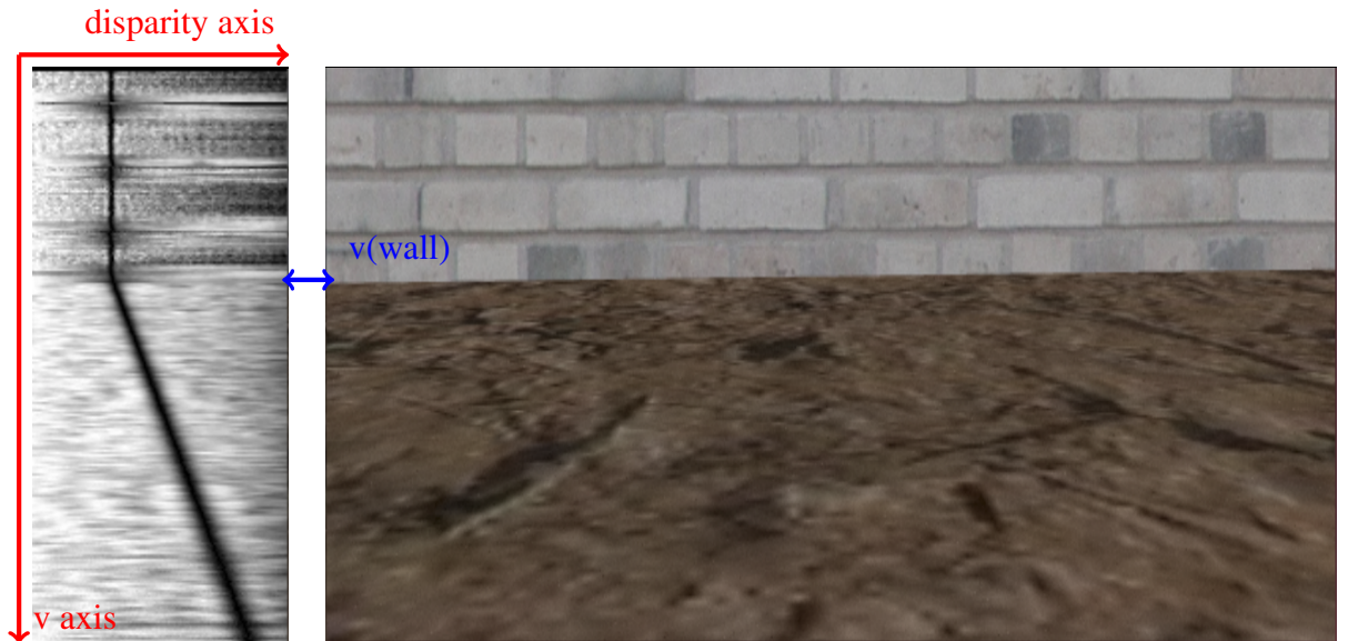
Figure 3.2: v -disparity representation and original image with a vertical wall present
