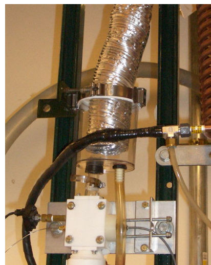
Figure 3.28 The water separator, a cross section drawing (left), photograph (right)
