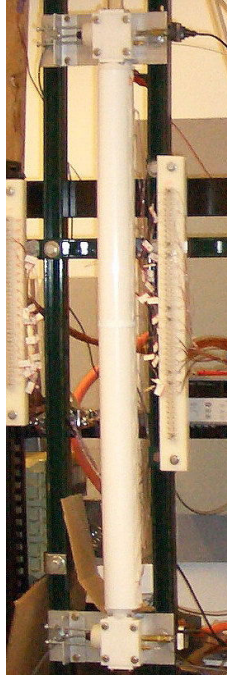
Figure 3.25 The insulated second cylindrical test section
