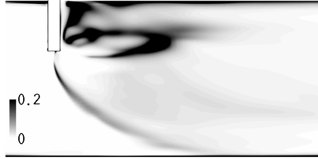
Figure 44: Time-averaged temperature profiles from the current LES and without turbulent model. The dotted line indicates the location of x - z cross section.
