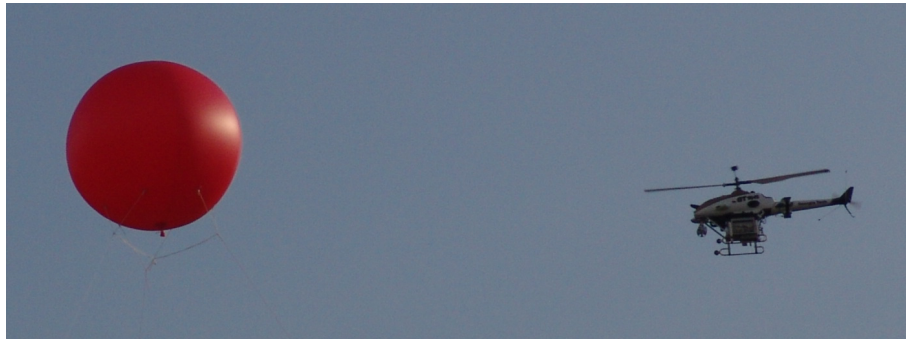
Figure 1: The GT Max UAV performing vision-based target tracking and obstacle avoidance using a weather balloon.
