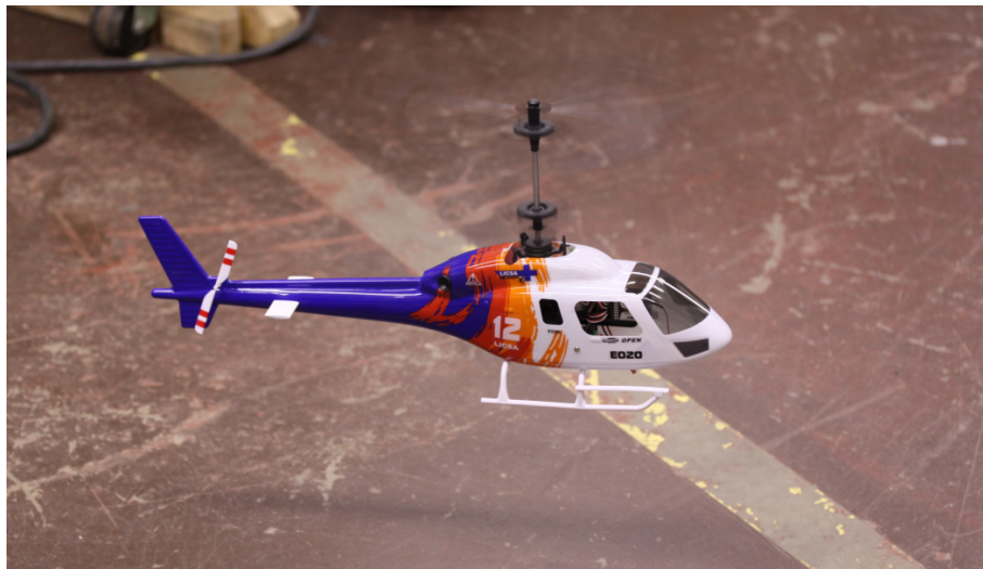
Figure 2: The E-Sky ® Big Lama. Photo courtesy Allen Wu. Note: the tail rotor on this aircraft is neither functional nor required.
