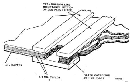
Figure 4: Diagram of W.C. Brown's Thin Film Etched Circuit Rectenna<sup>27</sup>
