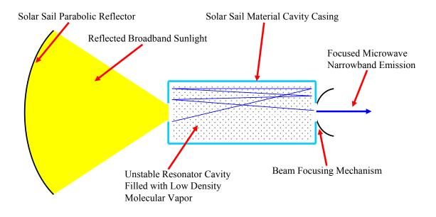
Figure 6: Solar pumped maser system concept diagram
