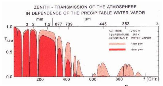
Figure 1: Atmospheric transmission as a function of frequency<sup>15</sup>
