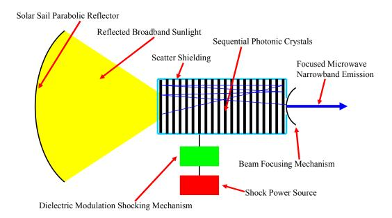
Figure 5: Shocked Photonic Crystal System Concept Diagram
