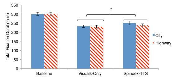
*Figure 10.* Graph of the dwell time on the primary task across drive type for the two experimental conditions and baseline. Higher bars represent more time eyes on the road. Standard error is shown via error bars and significant differences are marked with "\*".
