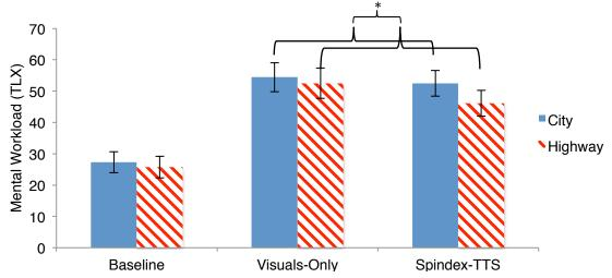
*Figure 12.* Graph of mental workload via NASA-TLX across drive type for the two experimental conditions and baseline. Higher bars represent more workload. Standard error is shown via error bars and significant differences are marked with "\*".
