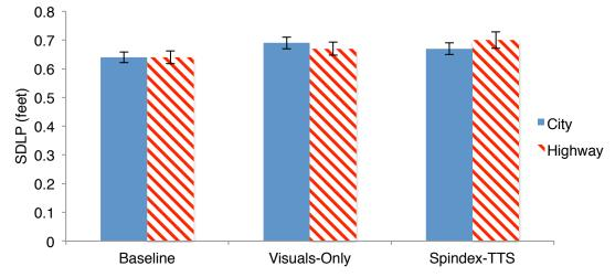
*Figure 8.* Graph of the standard deviation of lane position (SDLP) across drive type for the two experimental conditions and baseline. More deviation is representative of worse driving performance. Standard error is shown via error bars.
