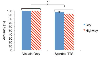
*Figure 6.* Graph of song finding accuracy across drive type for the two experimental conditions. Higher accuracy is visualized with higher bars. Standard error is shown via error bars and significant differences are marked with "\*".
