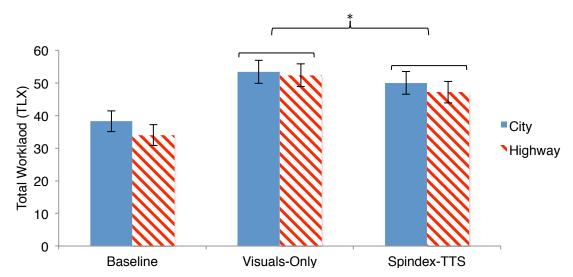
*Figure 13.* Graph of total workload via NASA-TLX across drive type for the two experimental conditions and baseline. Higher bars represent more workload. Standard error is shown via error bars and significant differences are marked with "\*".
