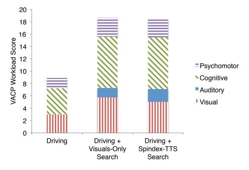
*Figure 16.* Graph of VACP ratings for each modality for the two experimental conditions and the baseline. The experimental condition values were determined by adding the driving averages across raters to the search task ratings averaged across rater.
