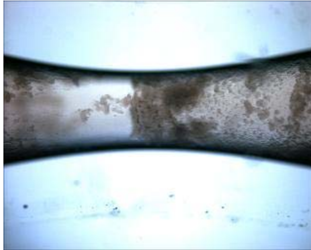
Figure 20B. 4x magnification at the throat of the stenosis showed that some surfaces were completely clear of thrombus which may have been removed in flow.
