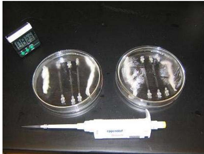
Figure 5. Collagen was coated in test sections by filling the sections and then letting them dry in a humid environment created by rolled paper towels soaked in hot water in a closed Petri dish.
