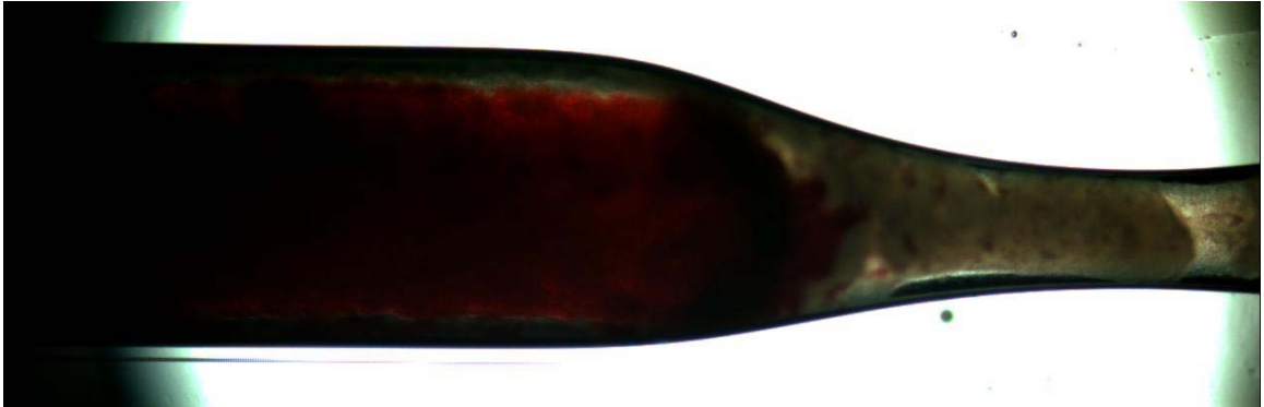
Figure 81. Upstream end of stenosis showed occluding thrombus before removal. Throat diameter was 610 \mu\text{m} . 2x magnification.
