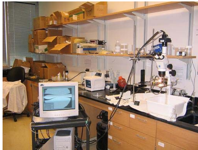
Figure 8. Image of thrombus formation visualization set up. A CCD camera on the microscope is attached to a computer with imaging software. Equipment photographed December 15, 2004.
