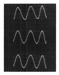
(c) Further detail of waveform of phase 1–2. Top-to-bottom: successive frames show successive cycles in the order 1–2–3, 3–4–5, 5–6–7. Note cycle-to-cycle variations.
