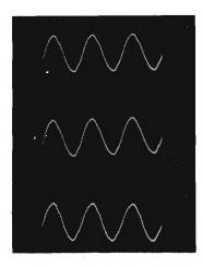
(a) Output voltage waveforms at full load, 0.8 power factor. Top-to-bottom: phase 3~1, phase 1-2, phase 2-3.
