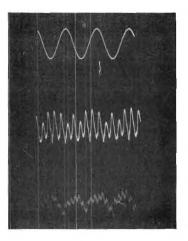
(d) Top: Output voltage wave with separately excited field. Full load, 0.8 power factor. Compare with 2(a).
