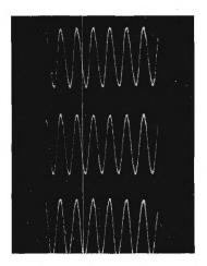
(b) Output voltage wave forms at full load, unity power factor. Top-to-bottom: phase 3-1, phase 1-2, phase 2-3. The fact that successive cycles are different is evidence that the distortion includes frequencies other than harmonics of 400 cycles.
