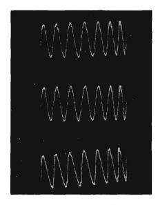
(a) Wave-forms at rated voltage, no load. Top-to-bottom: phase 3–1, phase 2–3, phase 1–2. Note variation in waveforms.
