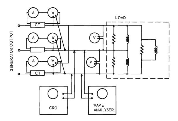
Figure 1. Schematic Diagram of Instrument Connections.
