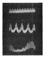
(c) Top: Field excitation voltage with output voltage set to 105 volts. Full load unity power factor.
