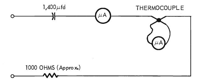
Figure 3. Thermocouple Voltmeter Circuit.
