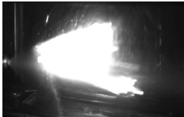
Figure 3.3-2. A sample image of a successful ignition event with room temperature fuel spray, with the camera exposure synchronized according to timing signals in Figure 3.1-1.
