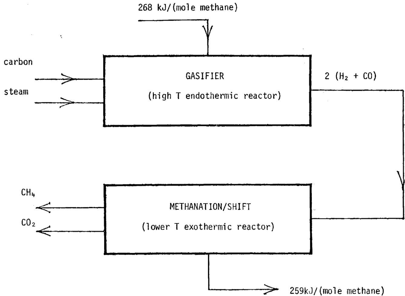
Figure 1: A Representative Candidate Process for a High-Temperature Heat Pump Application
