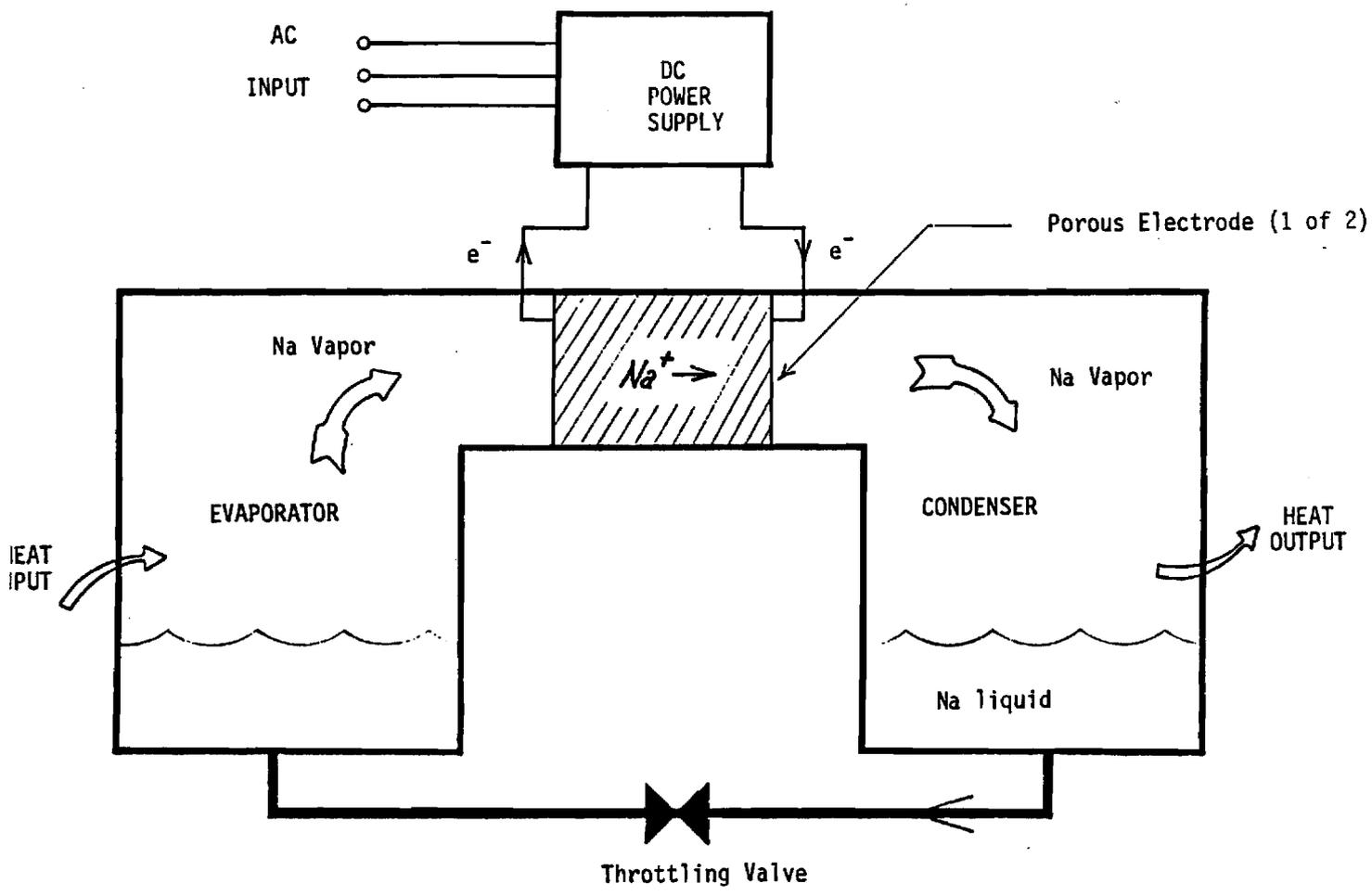
Figure 2. Schematic of High-Temperature Heat Pump Using Vapor Compression Cycle
