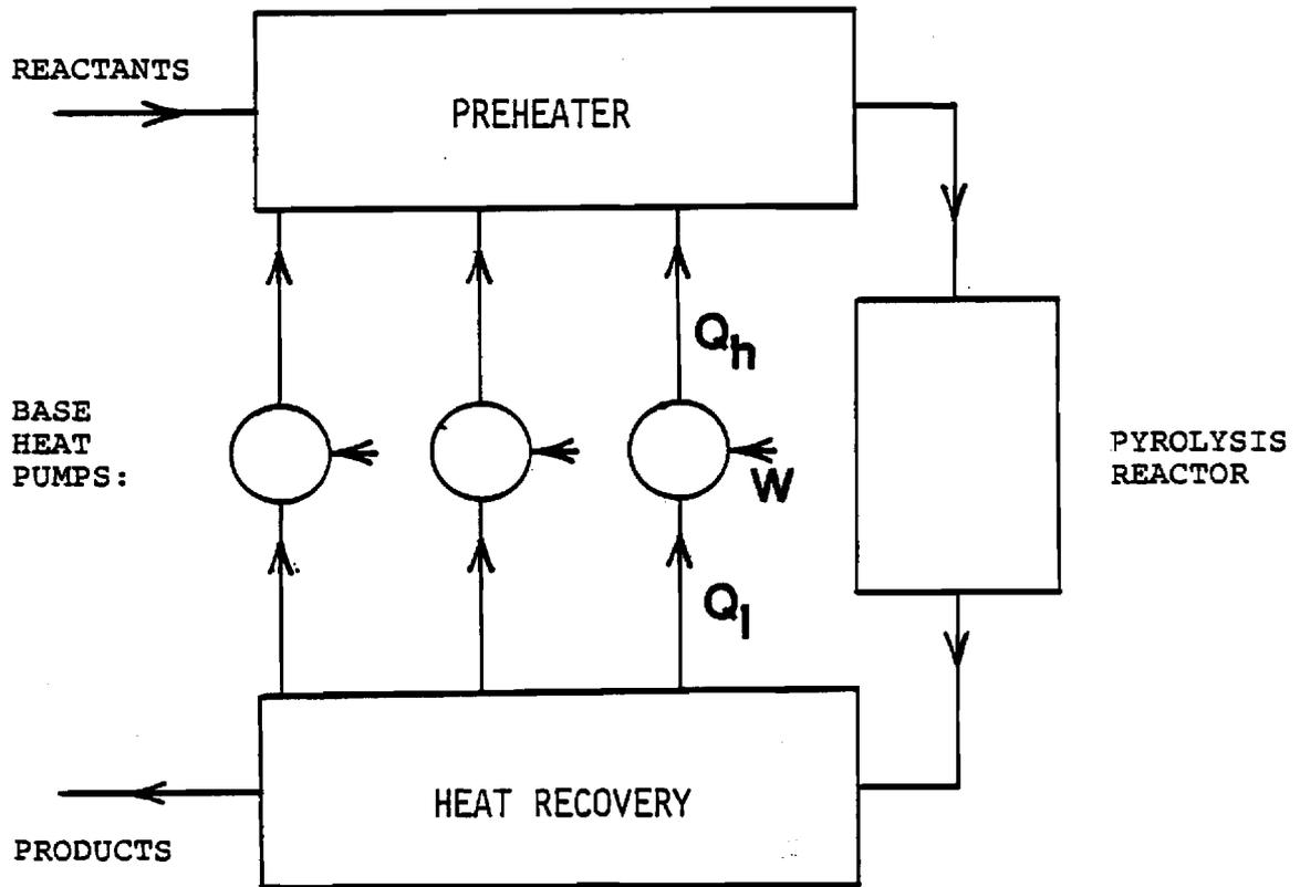
Figure 5. Schematic Simplified Plant for Ethylene Production Using High-Temperature Heat Pump
