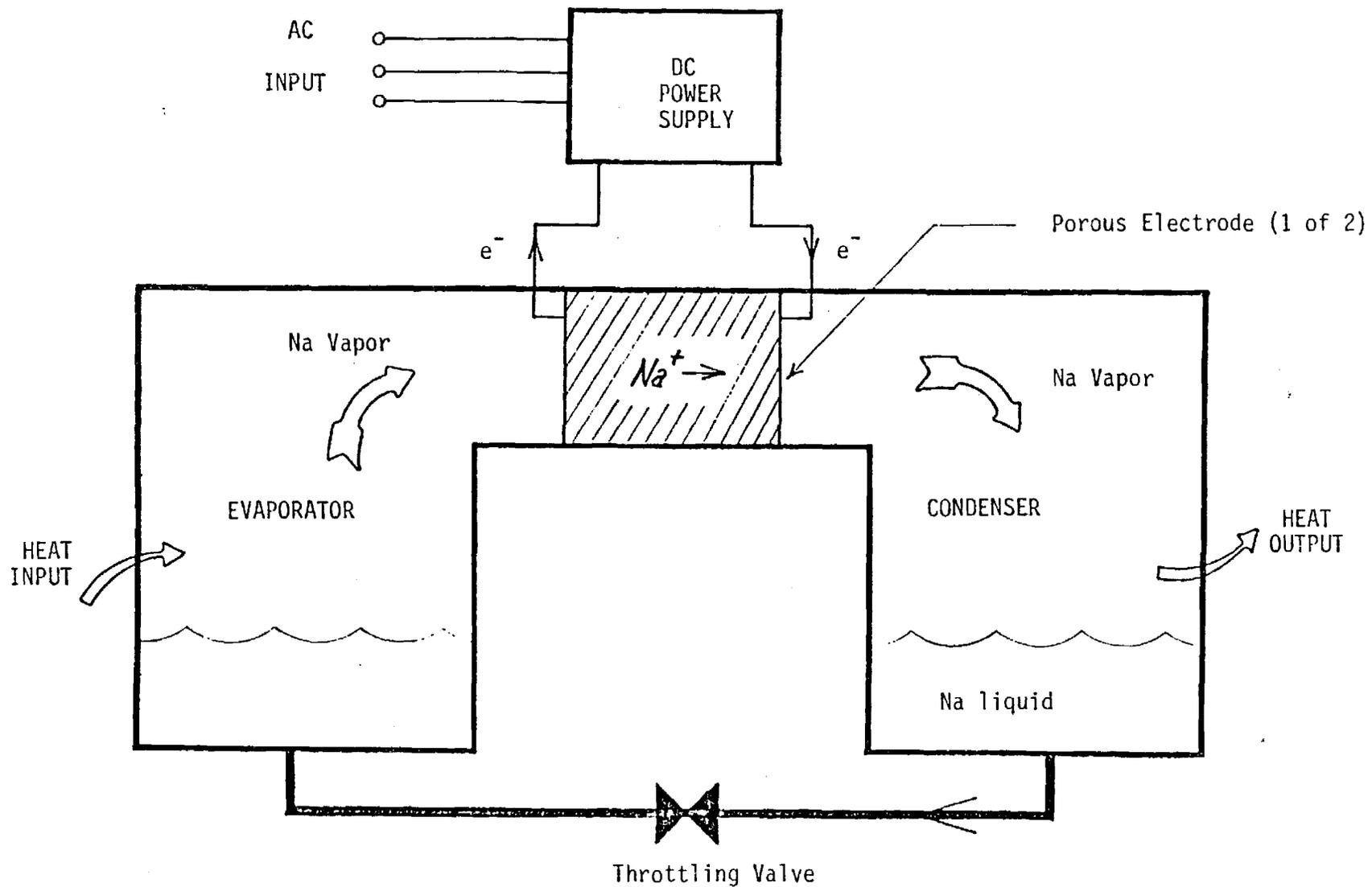
Figure 2: Schematic of High-Temperature Heat Pump
