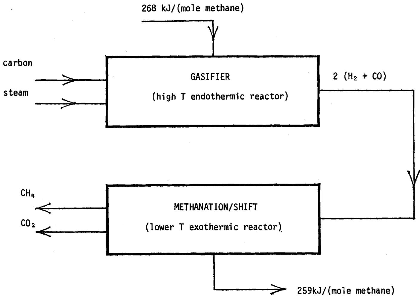
Figure 1 A Representative Candidate Process for a High-Temperature Heat Pump Application
