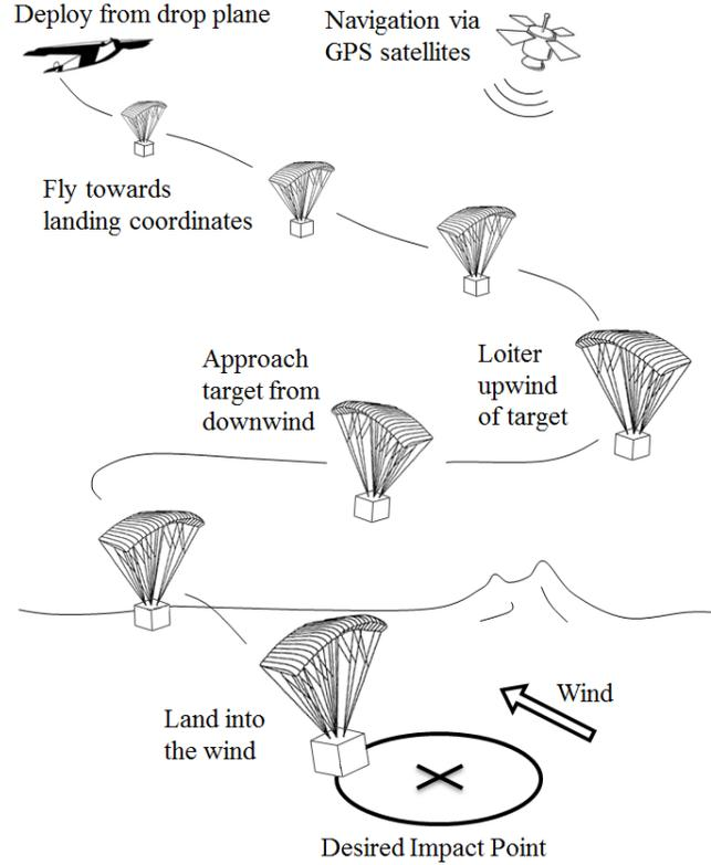
Figure 1.2: Typical flight profile for modern precision airdrop systems.
