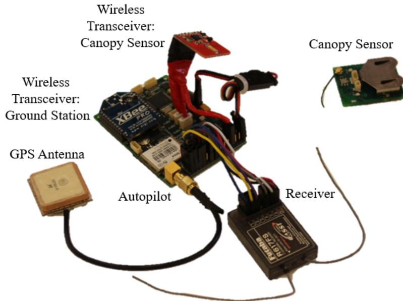
Figure 3.2: Flight electronics used in the small-scale precision airdrop system.
