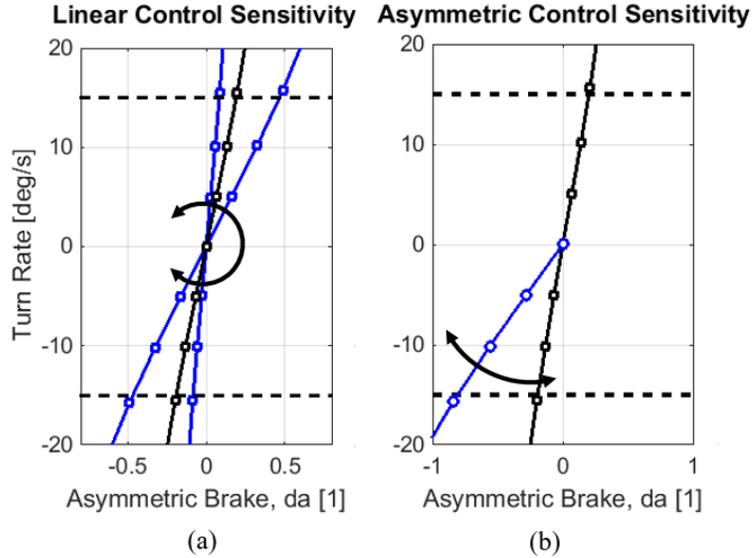
Figure 6.1: Depictions on how the control authority can be rotated (a) symmetrically and (b) asymmetrically to represent various types of degraded flight conditions.
