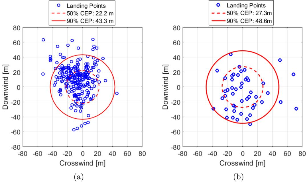
Figure 7.2: Landing dispersion of GPS based feedback algorithm in (a) simulation and (b) experimental flight testing.
