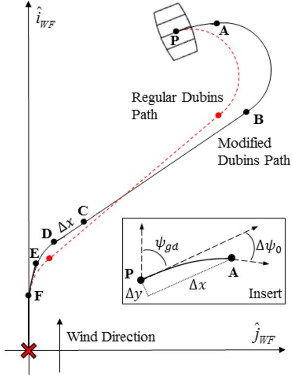
Figure 5.7: Comparison of regular and modified Dubins path planning algorithms.
