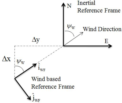
Figure 4.1: Visual representation of the wind based reference frame. It is offset from the inertial origin by an amount  $(\Delta x, \Delta y)$  and rotated to align with the wind direction.
