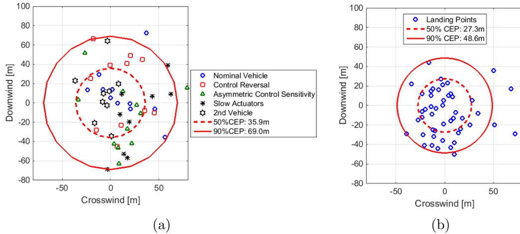
Figure 6.28: Experimental Landing results of the (a) Conventional GNC and (b) Hyperadaptive GNC algorithms.
