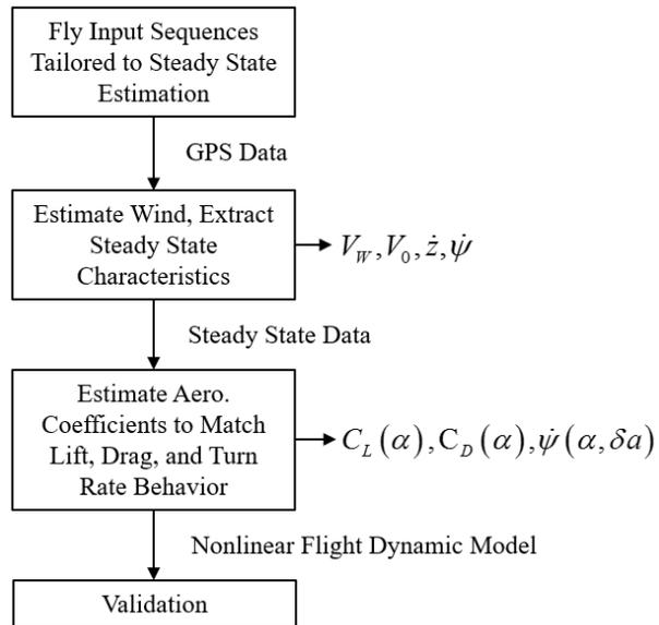
Figure 3.3: Strategy to characterize aerodynamic parameters from steady-state flight data [4].
