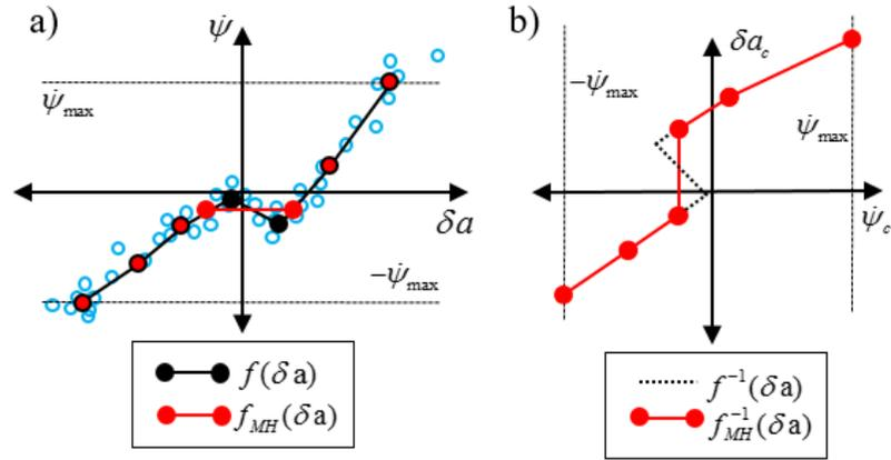
Figure 5.9: a) Graphical representation of the SNLM estimator; b) Control mapping characterized by the Map Handler.
