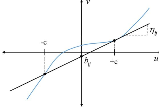
Figure 5.4: Linear approximation of an example SNLM under PRBS input.
