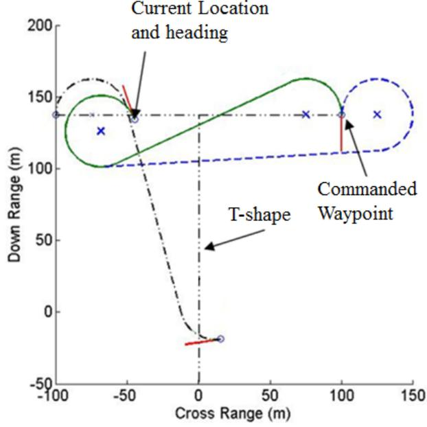
Figure 4.2: Visualization of Dubins path planning transitioning from the left waypoint to the right.
