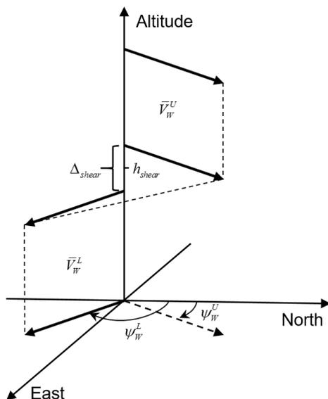
Figure 2.3: Horizontal wind shear profile.
