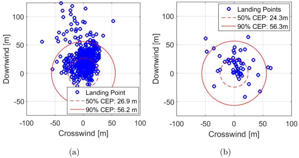
Figure 7.7: Results of the  $\{R, z\}$  beacon feedback method tested in (a) simulation and (b) experimental flight testing.
