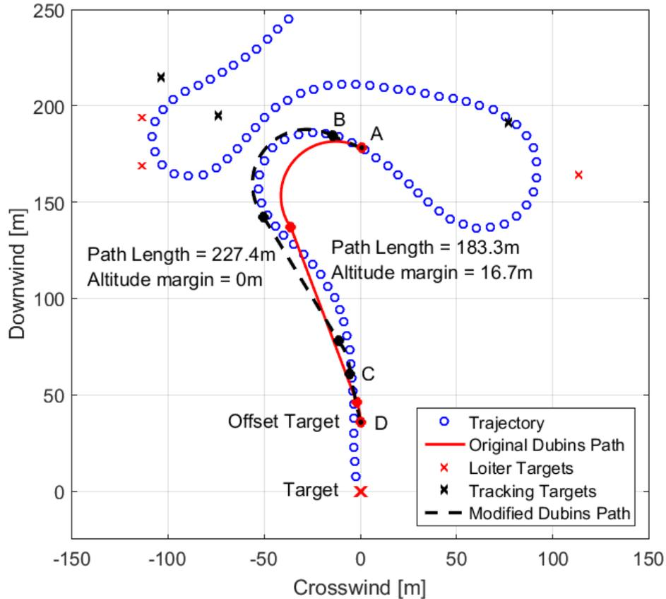
Figure 6.12: Simulation of the hyperadaptive GNC showing the modified Dubins paths used to calculate the flight distance to the offset target.
