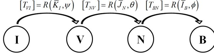
Figure 2.2: Graphic representation of the 3-2-1 Euler transformation from Inertial to Body reference frames.
