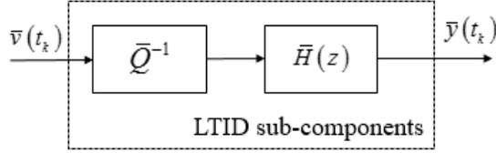
Figure 5.5: Decomposed realization of the LTID block under PRBS input.
