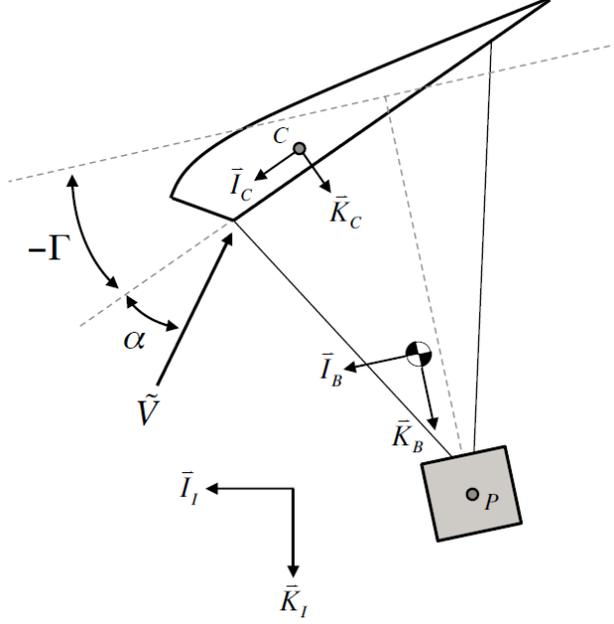
Figure 2.1: 2D representation of a parafoil and payload system
