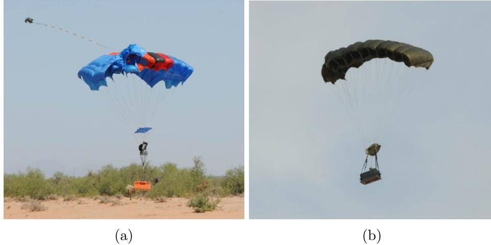
Figure 1.4: Autonomous airdrop system with ripped (a) upper surface canopy and (b) right canopy cells caused by high shock loading during inflation [3].
