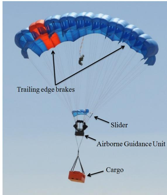
Figure 1.3: Modern guided, ram-air parafoil.
