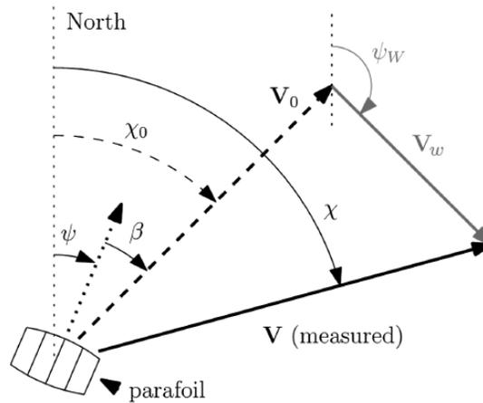
Figure 3.4: Vector diagram illustrating the combined vehicle and atmospheric velocities [4].
