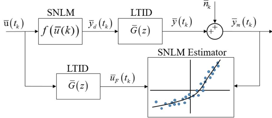
Figure 5.6: Representation of method used to generate a real-time comparison of the input-output relations.
