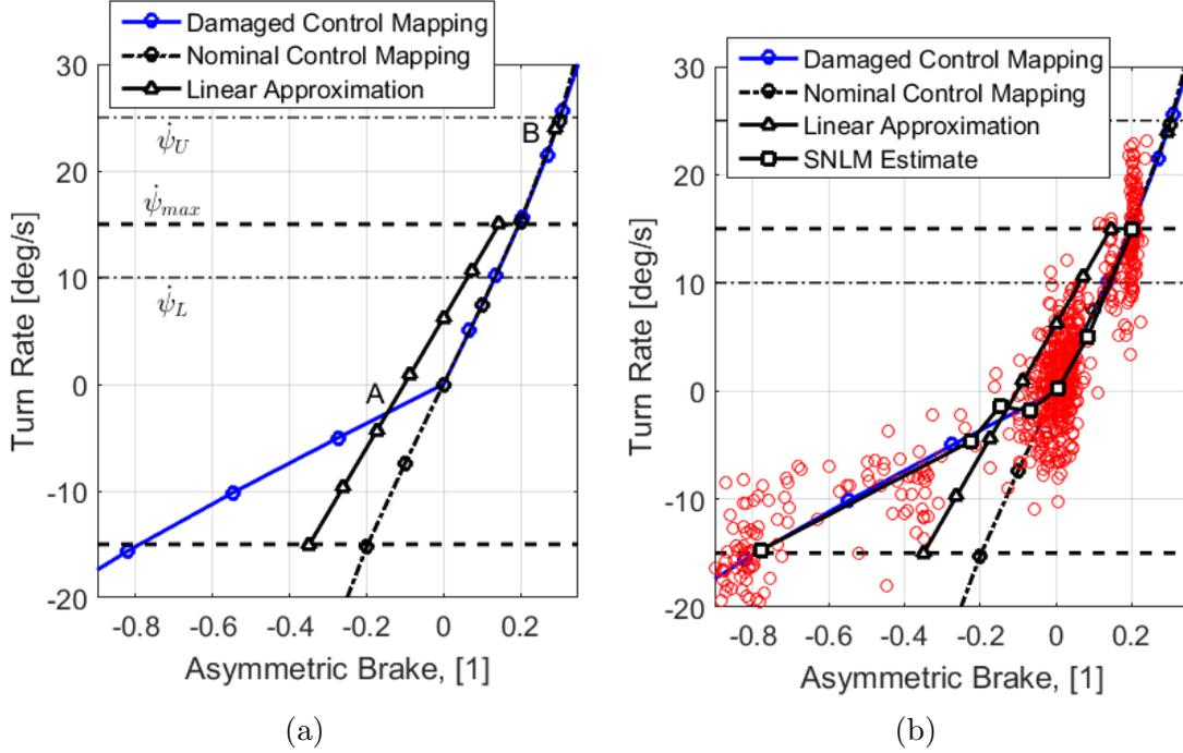
Figure 6.5: SNLM Estimate for a vehicle with asymmetric turn rate response after (a) estimation of the LTID parameters and (b) the conclusion of the flight.
