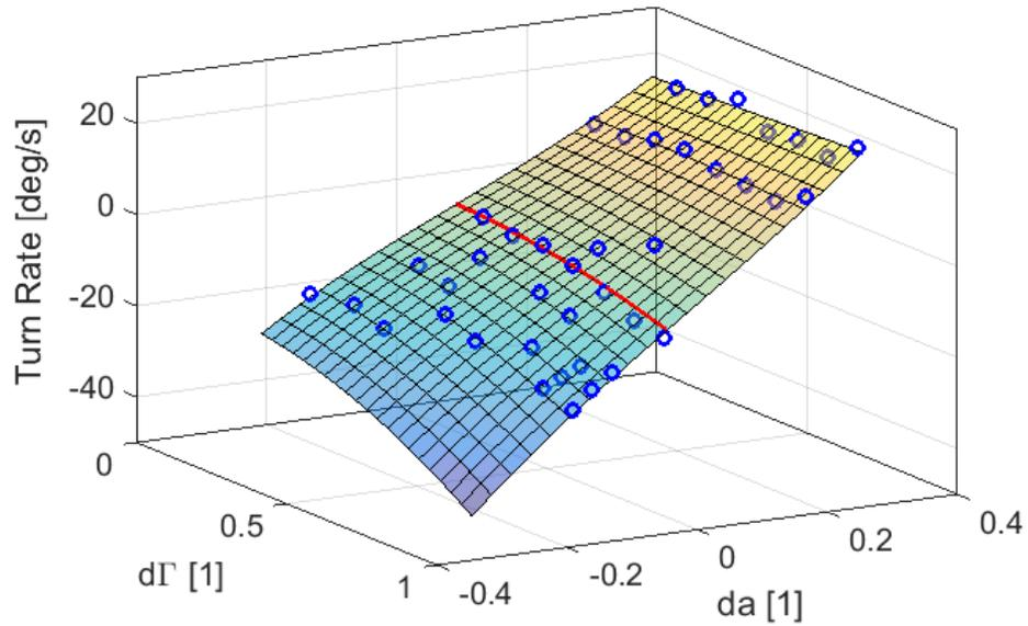
Figure 3.6: Lateral performance of the small-scale airdrop vehicle. Dots represent experimental measurements and the surface is a 2nd order fit of the data.
