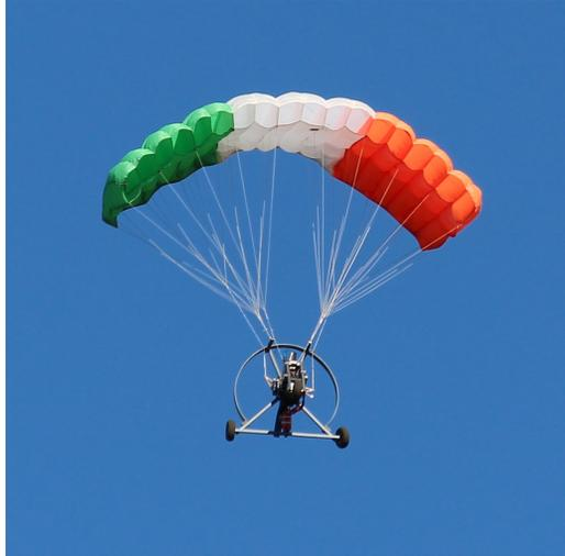
Figure 6.27: Second parafoil and payload system used to flight test the hyperadaptive GNC. Termed the Irish canopy due to the color selection.
