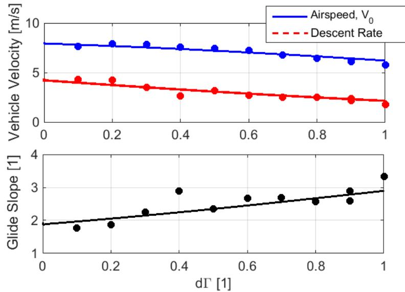
Figure 3.7: Longitudinal performance of a small-scale airdrop system. Dots denote experimental measurements and lines are simulation results.
