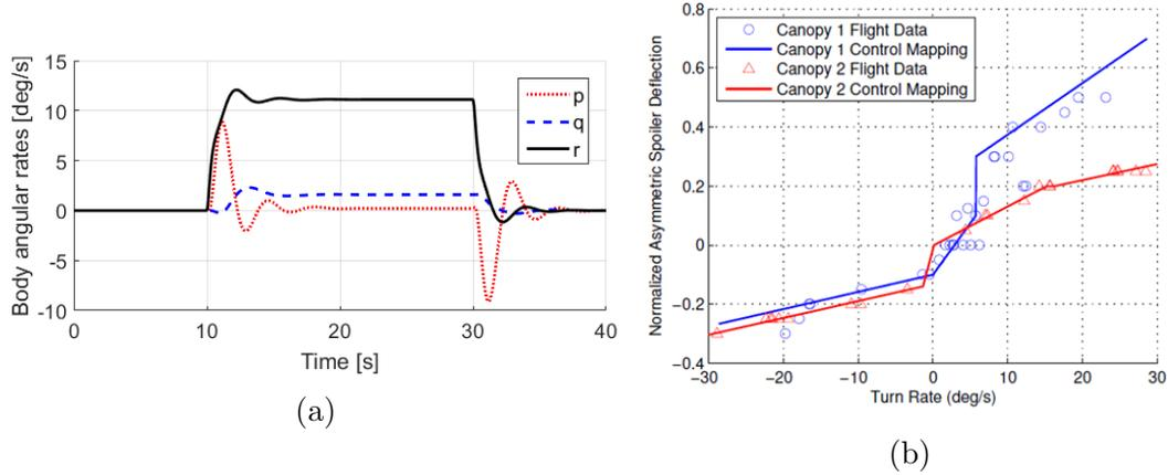
Figure 5.2: (a) Simulated parafoil dynamic response to a step asymmetric brake input commanded at  $t = 40$  sec; (b) Identified control mappings from flight testing of two  $20 \text{ ft}^2$  canopies [5].
