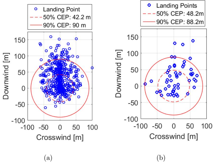
Figure 7.5: Landing dispersion of the  $\{\psi_B, z\}$  feedback algorithm based on (a) simulation results and (b) experimental flight testing.
