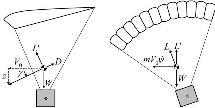
Figure 3.5: Decomposition of lift and drag forces for a parafoil in a steady turn [5].
