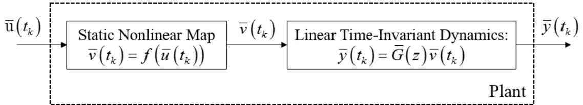
Figure 5.3: Graphic representation of a Hammerstein Model.
