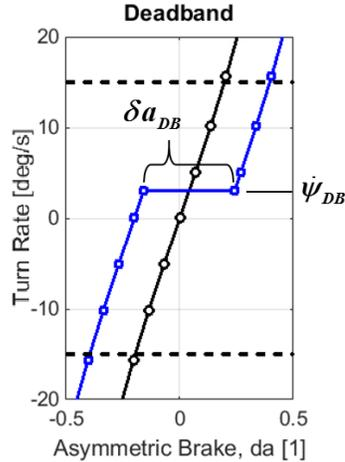
Figure 6.14: Nonlinear mapping that introduces a deadband of width  $\delta a_{DB}$  at a given turn rate  $\dot{\psi}_{DB}$ .
