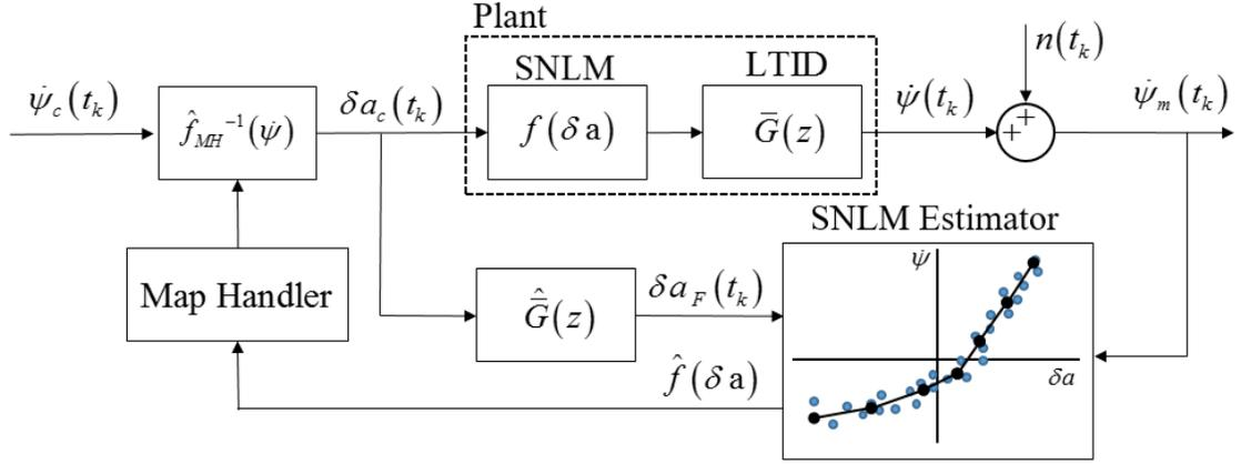
Figure 5.8: Block diagram representation of the control strategy used in the hyper-adaptive GNC.
