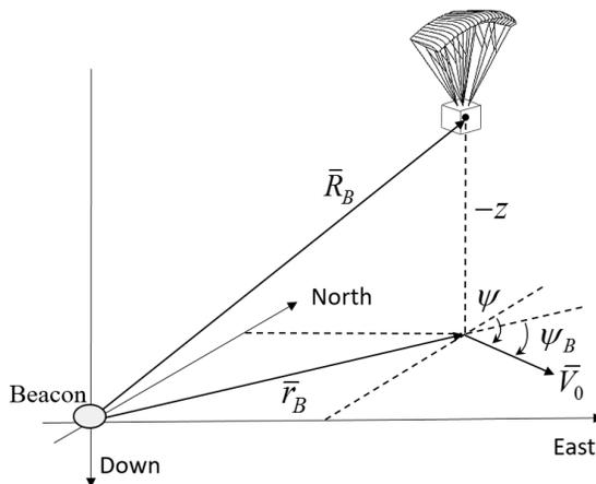
Figure 7.1: Spherical polar representation of the drop zone for beacon feedback control.
