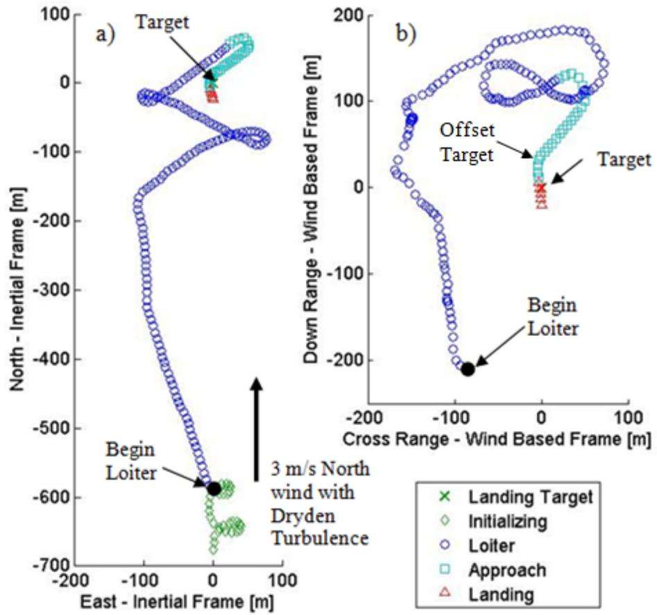
Figure 4.3: Example trajectory of an autonomous airdrop system plotted in the (a) inertial and (b) wind relative reference frames.
