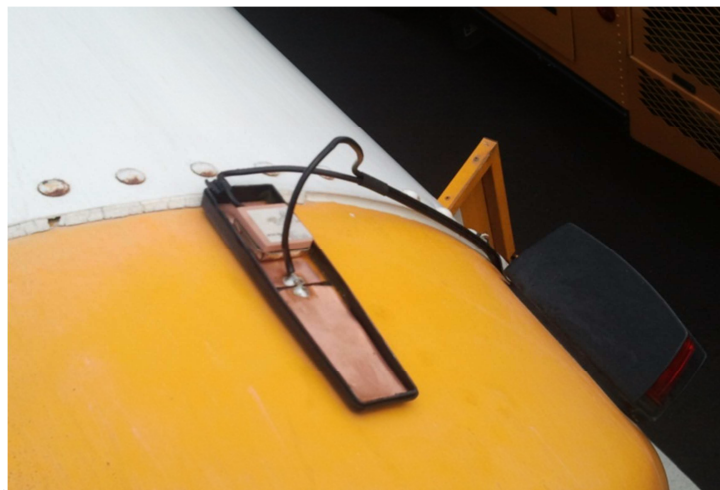
Figure 3.14: Example of a Broken Cellular Antenna
