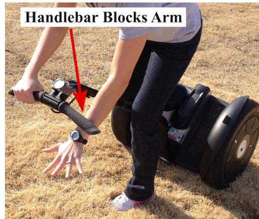
Figure 119: Segway handlebar blocking rider's arm.
