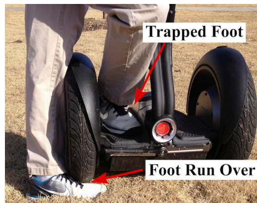
Figure 117: Rider's feet trapped by wheel.
