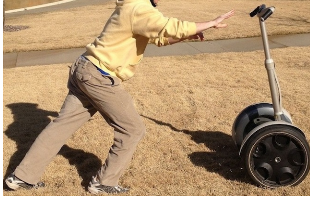
Figure 118: Segway moving without a rider in balance mode.
