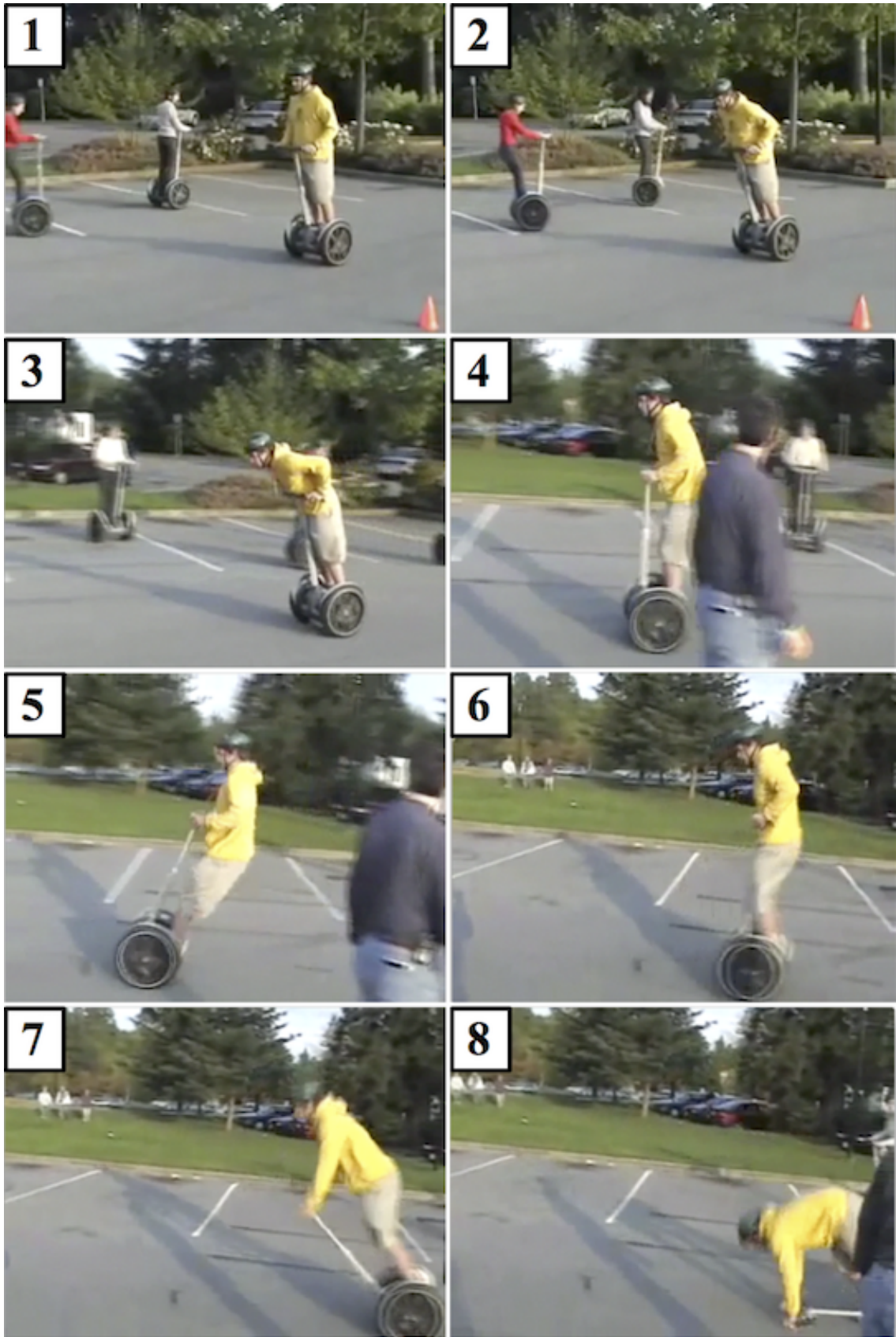
Figure 3: Sequence of video frames showing Segway rider oscillation and crash [60].
