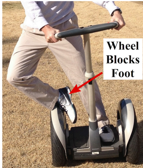
Figure 116: Segway right wheel blocking rider's foot.
