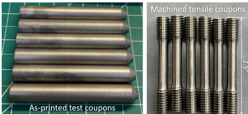
Figure 20. Tensile coupons shown as printed and after machining.
