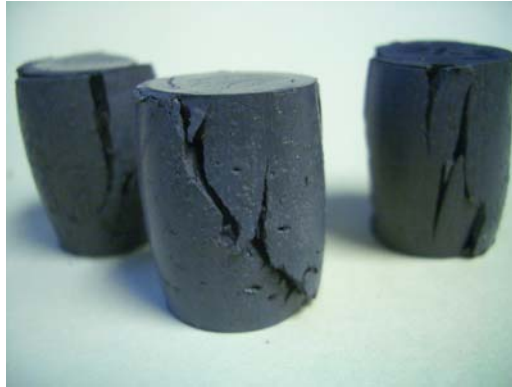
Figure 4-16: Photograph of Ni+nano Al+30wt% epoxy samples after compression testing. These show typical characteristics of the cast samples after compression tests.
