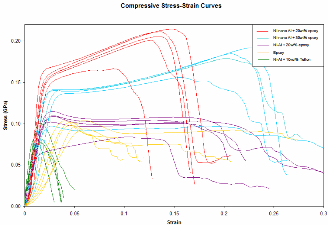
Figure 4-14: Stress-Strain curves generated during compression testing. The Ni+nano Al+20wt% epoxy samples (red curves) show the most superior static mechanical behavior in that they displayed the highest Elastic Modulus and compressive yield strength.
