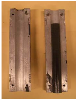
Figure 3-4: Photograph of Ni-Al + epoxy sample in open mold after curing.
