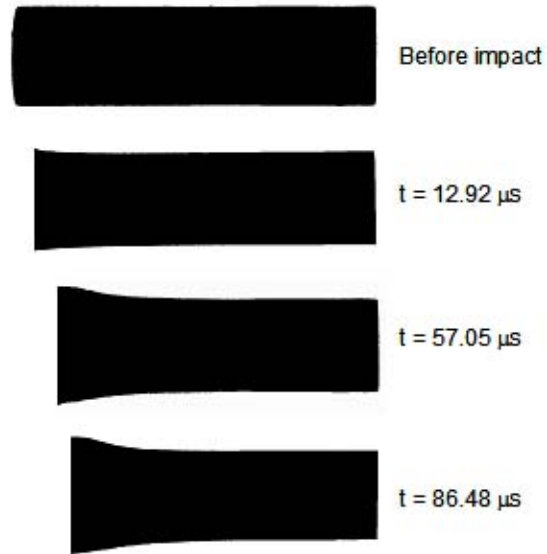
Figure 4-34: Deformation profiles used in House Analysis of Ni+nano Al+20wt% epoxy sample impacted at 100 m/s in shot 0430.
