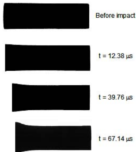
Figure 4-39: Deformation profiles used in House Analysis of Ni+nano Al+30wt% epoxy shot sample impacted at 100 m/s in shot 0431.
