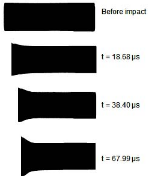
Figure 4-24: Deformation profiles used in House Analysis of pure epoxy sample impacted at 152 m/s in shot 0501.
