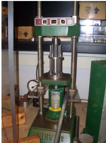
Figure 3-2: Photograph of 1/4" die in Carver Press.
