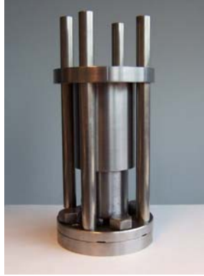
Figure 3-1: Photograph of 1/4" die in closed position.
