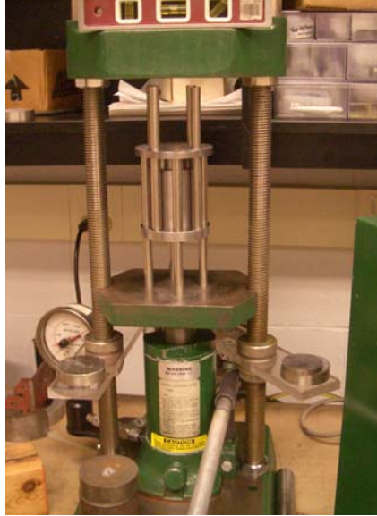
Figure 3-3: Photograph of 1/4" die with all 8 guide rods used to open die.
