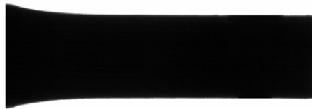
Figure 3-9: The profile of the deforming sample shown in Figure 3-8 isolated in Photoshop for use in the House analysis.
