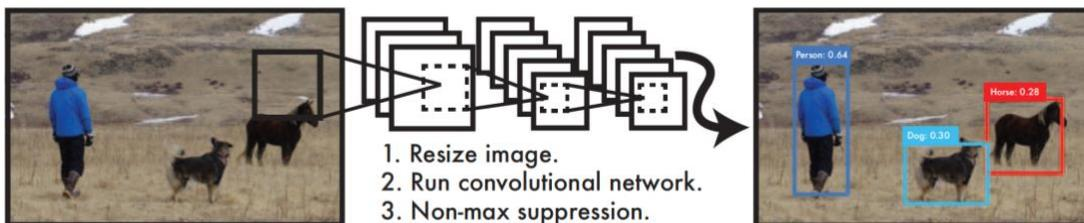
Figure 8: Object detection with YOLO
