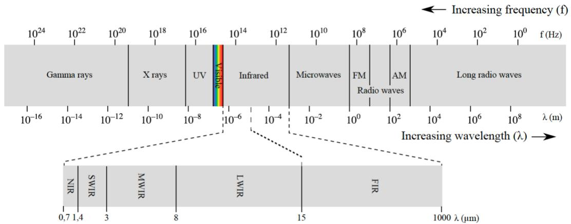
Figure 23: Electromagnetic spectrum with subdivided infrared range
