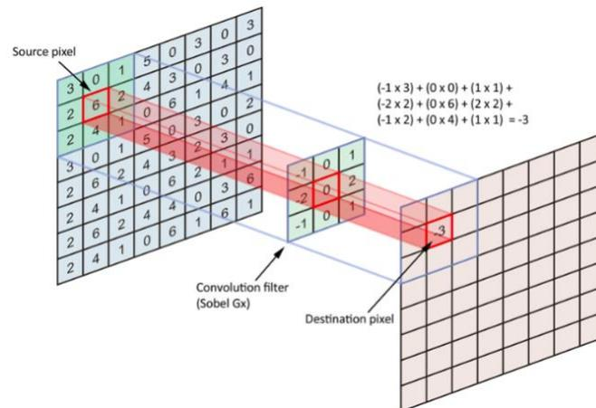
Figure 12: Filter application to source image in CNNs
