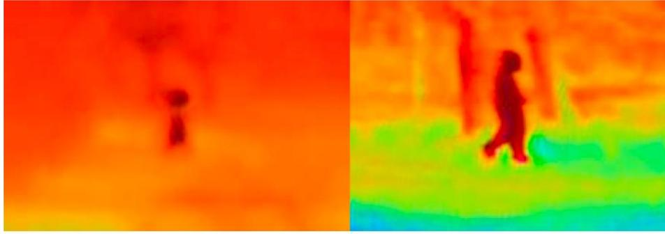
*Figure 24: A human recorded with standard lens at a distance of 110 m (left) vs. telephoto lens recorded at 165 m (right)*
