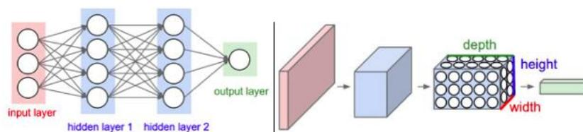
Figure 13: Regular Neural Network (left) compared to Convolutional Neural Networks (right)
