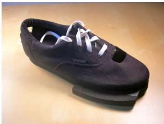
Figure 24. Shoe prototypes with flare and windows to accommodate markers
