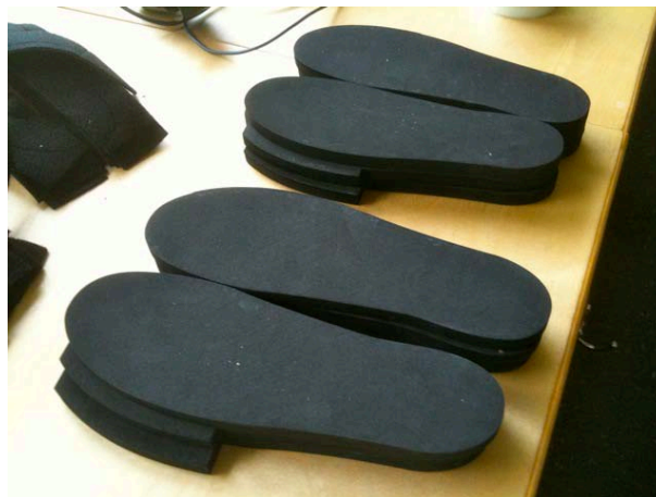
Figure 20. Sole Designs from laser cutter
