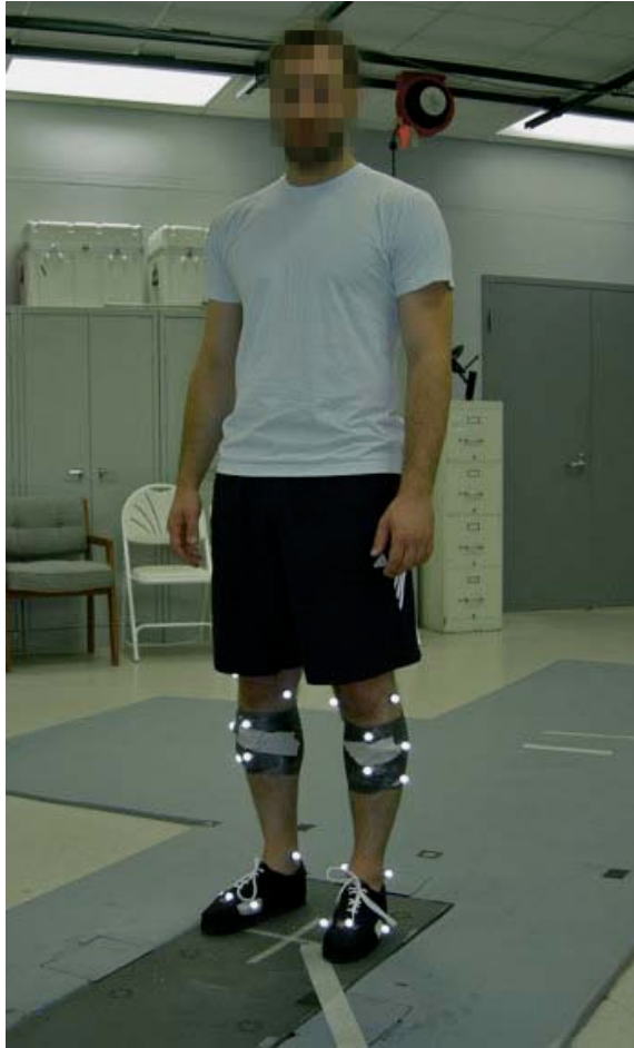
Figure 23. Reflective marker set used to capture ankle kinematic data
