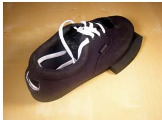
Figure 24. Shoe prototypes with flare and windows to accommodate markers
