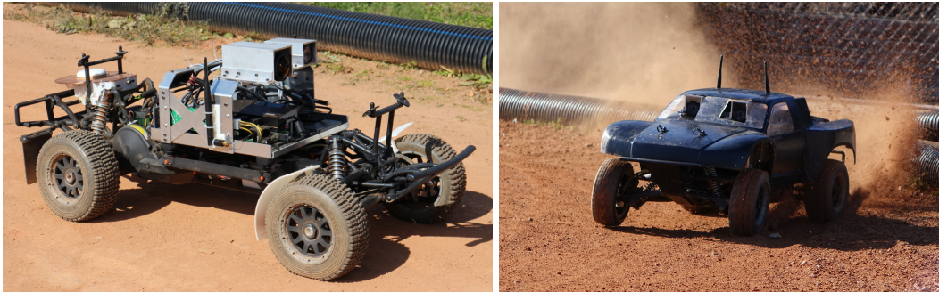
Figure 3.3: (Left) The AutoRally platform with onboard sensing and computing. (Right) The AutoRally platform performing a high speed maneuver.
