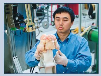
also constructed and tested a two-axis system with a servo control blade to perform all of the cutting motions. They further made progress on modeling the wing manipulation and cutting task. This work is critical to controlling the cutting path and optimizing yield.
