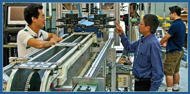
The automatic intelligent transfer system project focused on taking live birds on a moving conveyor belt and ordering them into singulated, properly oriented positions to be grasped by the device's proprietary grasping system.
