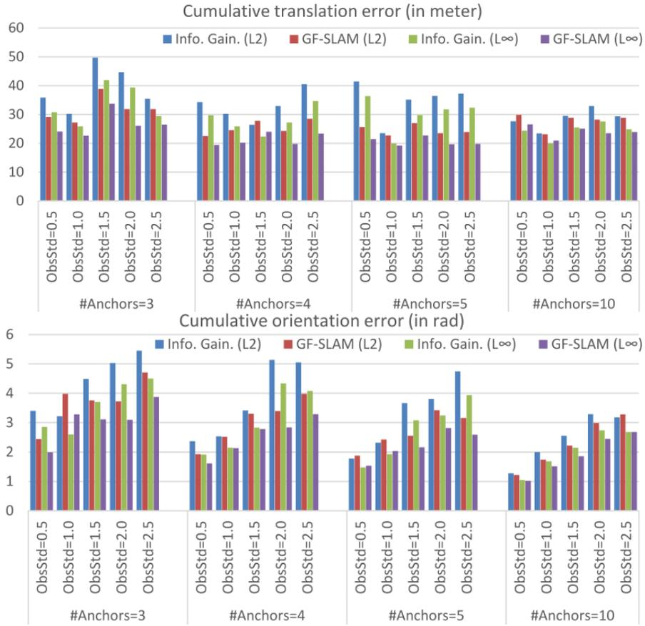
**Figure 28:** Results of simulation scenario #1 with cumulative translation errors and cumulative orientation errors. “ObsStd” stands for the standard deviation of observation noise in pixel units.
