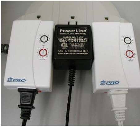
Figure 1: X10 components used in constructing a RWI. The black box is the Powerline interface that allows a computer to send signals via the serial port through the power lines. The white boxes are X10 receivers into which appliances can be plugged. Each receiver should have a different code, with up to 256 different codes available.
