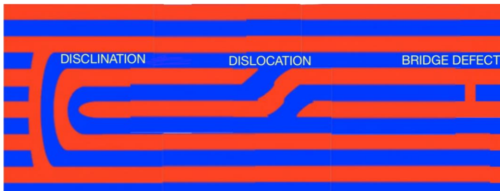
Figure 1-4 Directed Self-Assembly of Block Copolymers Defect Types
