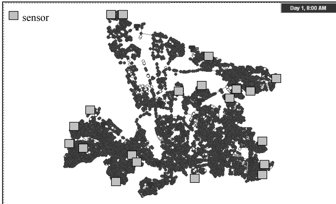
Figure 7.5 Optimal sensor locations with M = 20 for maximizing detection likelihood in the case of 2 nodes injected at 1 time for the Toms River WDS.
