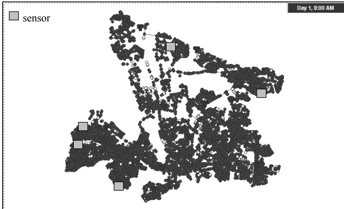
Figure 7.1 Optimal sensor locations with M = 5 for maximizing detection likelihood in the default attack case for the Toms River WDS.
