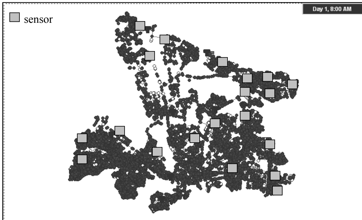
Figure 7.10 Optimal sensor locations with M = 20 for minimizing expected detection time in the default attack case for the Toms River WDS.
