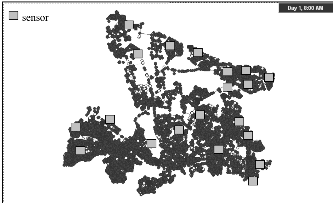
Figure 7.13 Optimal sensor locations with M = 20 for minimizing expected detection time in the case of 2 nodes injected at 1 time for the Toms River WDS.
