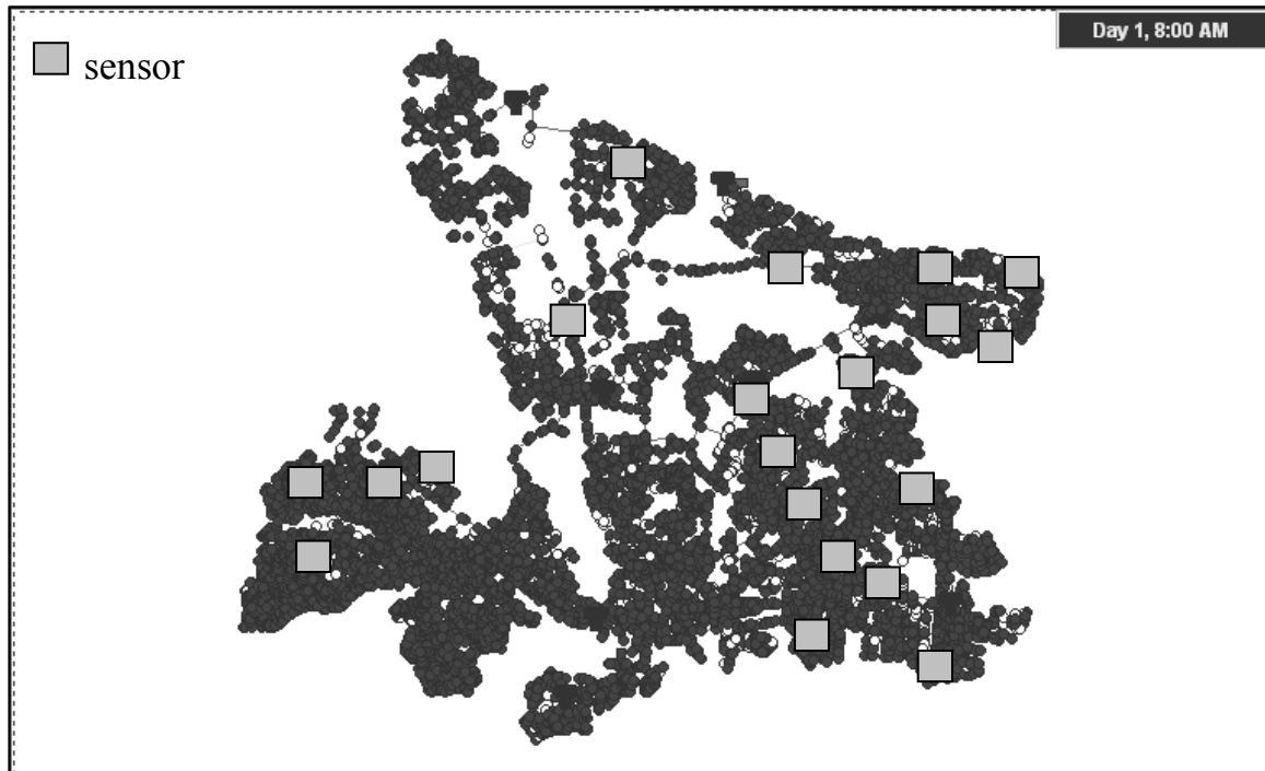
Figure 7.32 Optimal sensor locations with M = 20 for the three-prong multiobjective problem in the case of 2 nodes injected at 1 time for the Toms River WDS.
