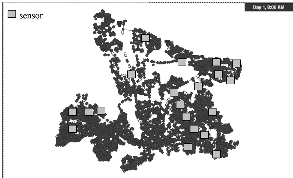
Figure 7.33 Optimal sensor locations with M = 20 for the three-prong multiobjective problem in the case of 2 nodes injected at 2 times for the Toms River WDS.
