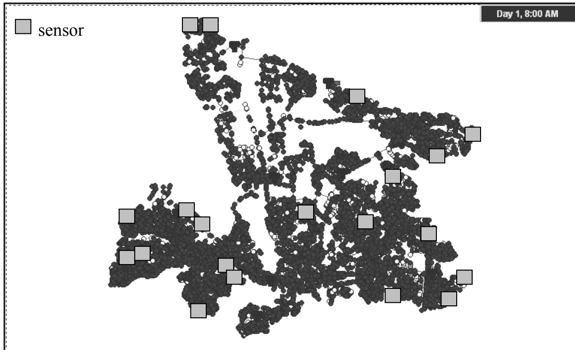
Figure 7.3 Optimal sensor locations with M = 20 for maximizing detection likelihood in the case of a detection resolution of 0.3 mg/L for the Toms River WDS.
