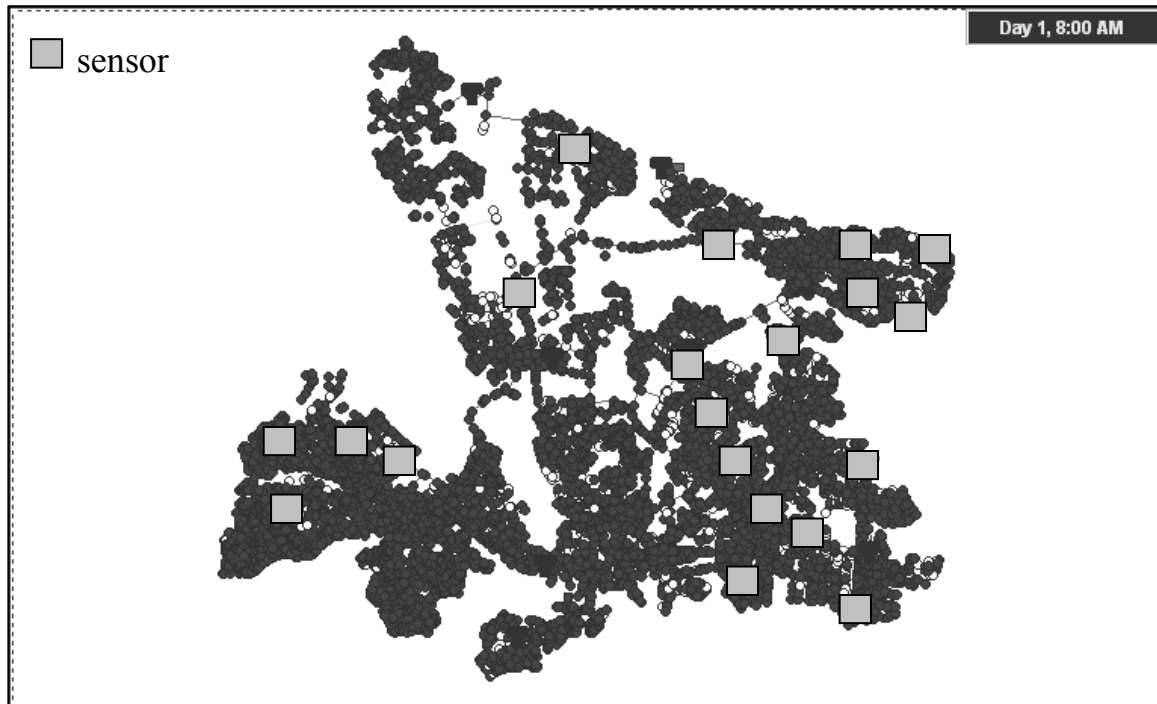
Figure 7.27 Optimal sensor locations with M = 20 for the three-prong multiobjective problem in the default attack case for the Toms River WDS.
