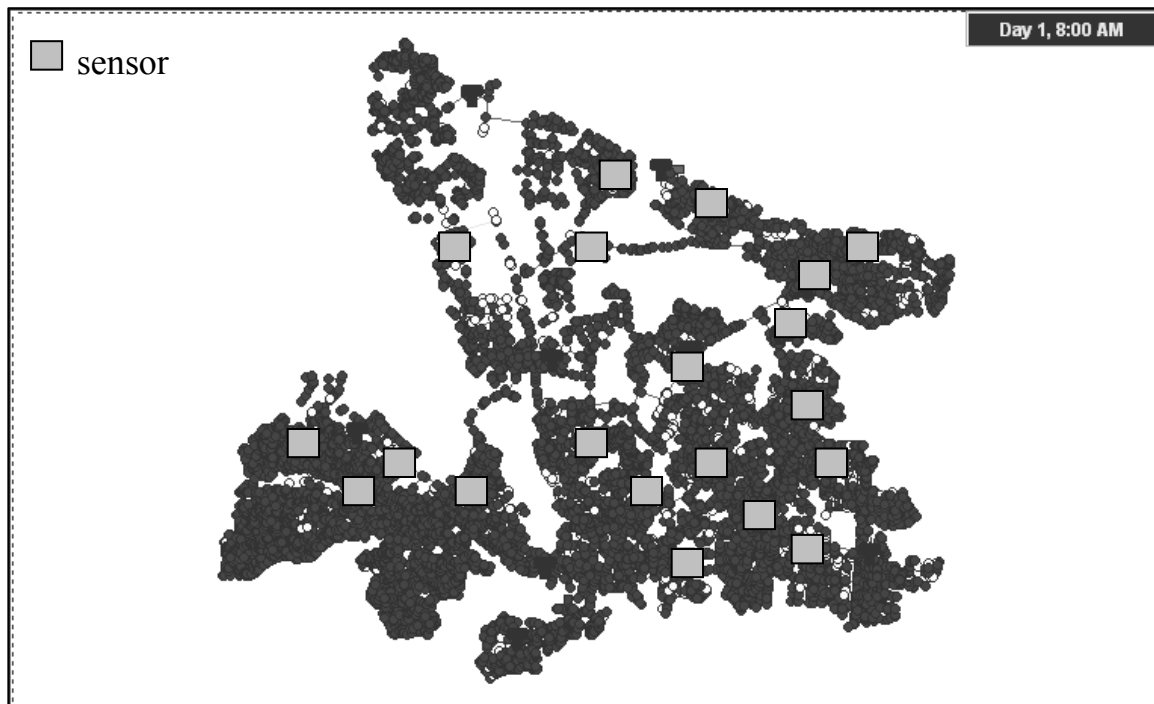
Figure 7.21 Optimal sensor locations with M = 20 for minimizing expected contaminated demand volume in the case of a hazard threshold of 0.0 mg/L for the Toms River WDS.
