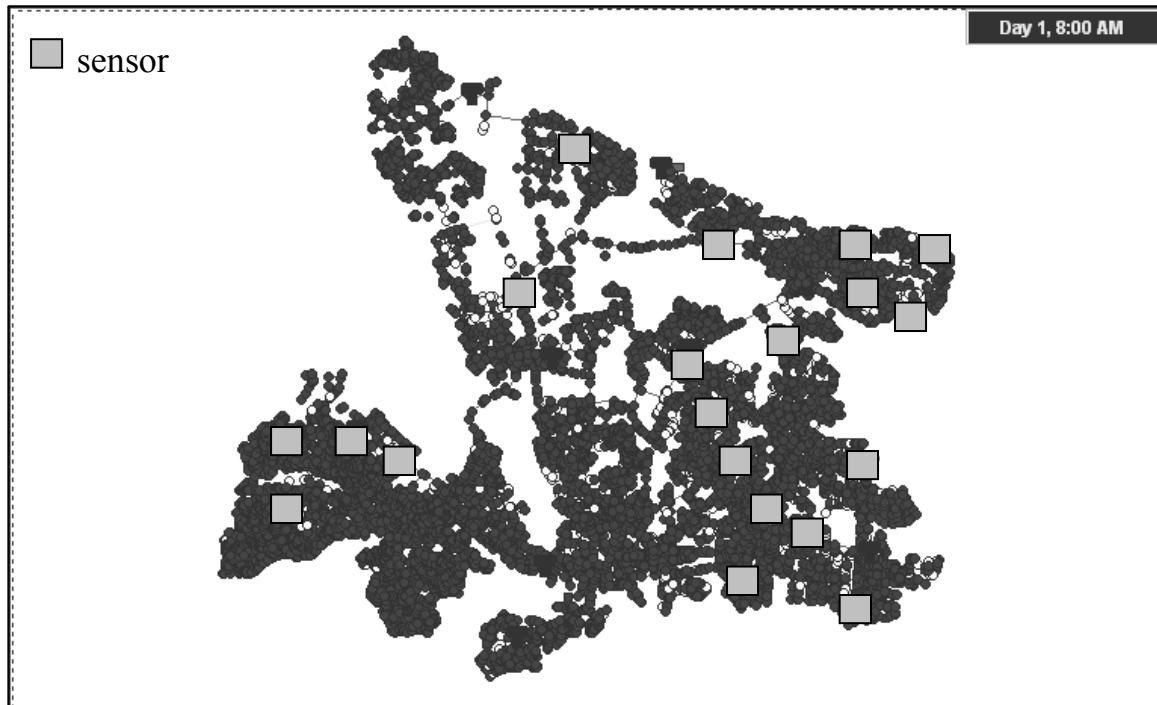
Figure 7.30 Optimal sensor locations with M = 20 for the three-prong multiobjective problem in the case of a hazard threshold of 0.0 mg/L for the Toms River WDS.
