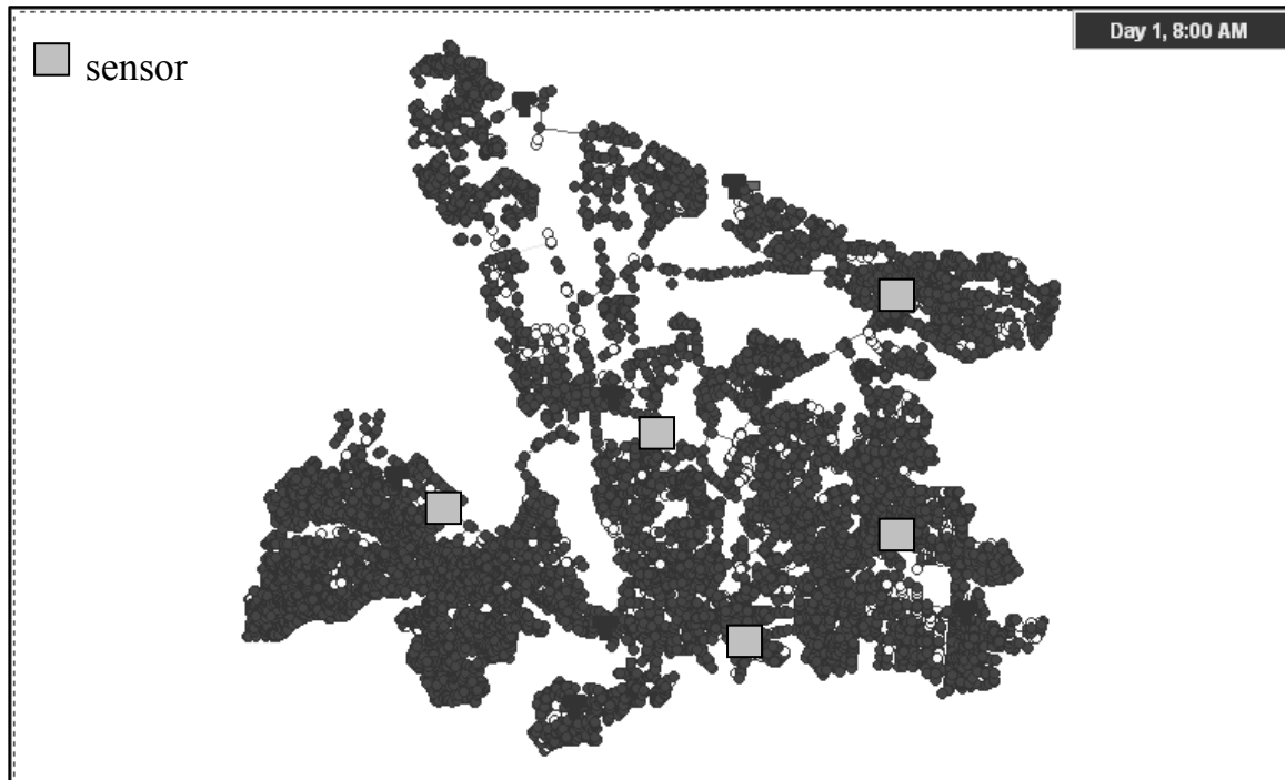
Figure 7.17 Optimal sensor locations with M = 5 for minimizing expected contaminated demand volume in the default attack case for the Toms River WDS.
