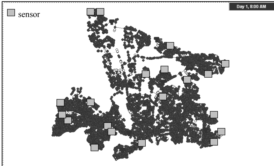
Figure 7.2 Optimal sensor locations with M = 20 for maximizing detection likelihood in the default attack case for the Toms River WDS.
