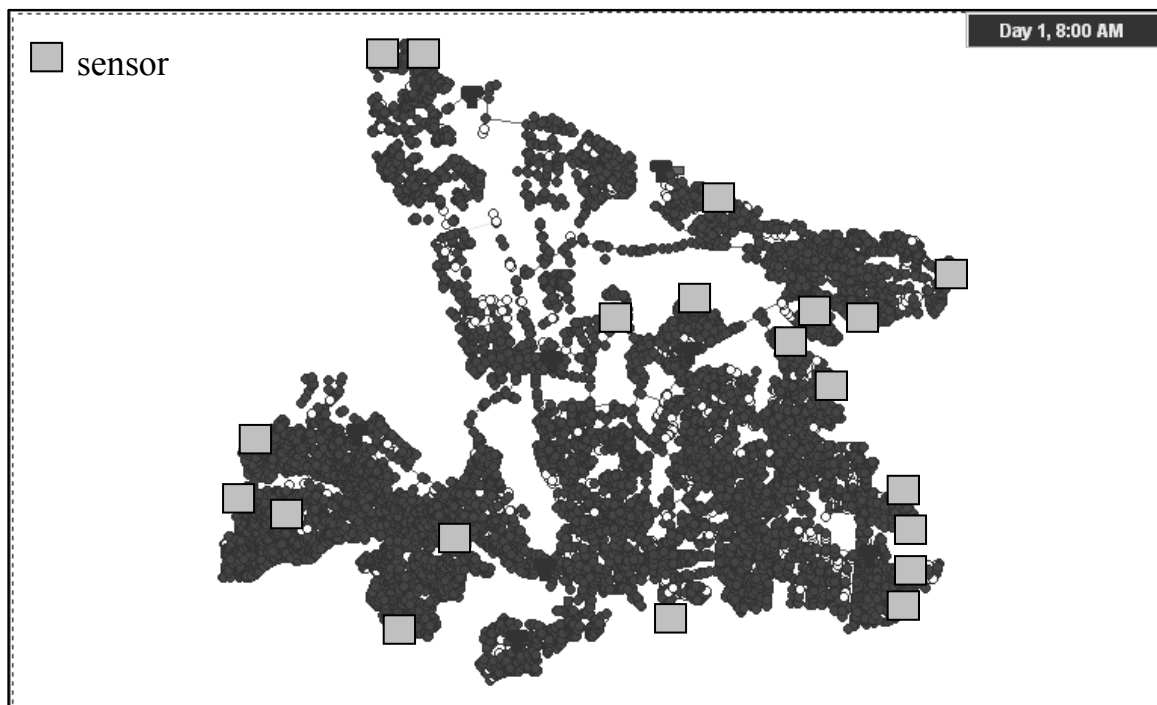
Figure 7.6 Optimal sensor locations with M = 20 for maximizing detection likelihood in the case of 2 nodes injected at 2 times for the Toms River WDS.
