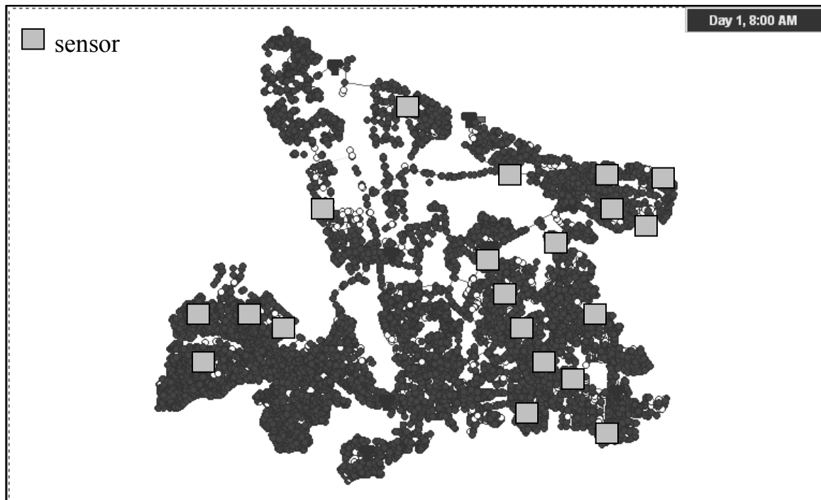
Figure 7.29 Optimal sensor locations with M = 20 for the three-prong multiobjective problem in the case of a 10-hour injection duration for the Toms River WDS.
