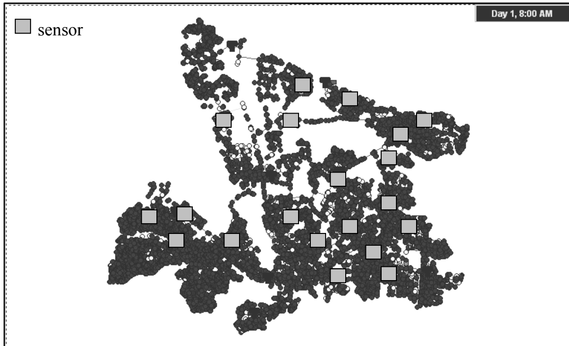
Figure 7.20 Optimal sensor locations with M = 20 for minimizing expected contaminated demand volume in the case of a 10-hour injection duration for the Toms River WDS.
