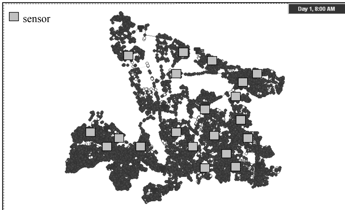
Figure 7.22 Optimal sensor locations with M = 20 for minimizing expected contaminated demand volume in the case of a 3-hour response delay for the Toms River WDS.
