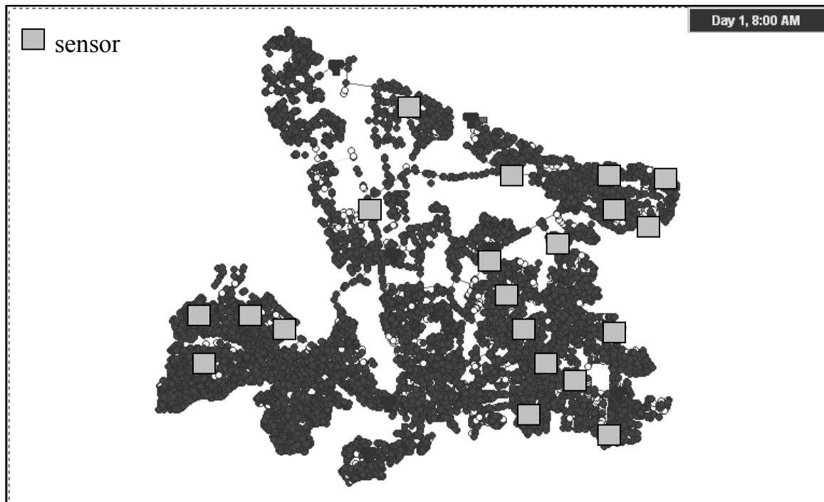
Figure 7.31 Optimal sensor locations with M = 20 for the three-prong multiobjective problem in the case of a 3-hour response delay for the Toms River WDS.
