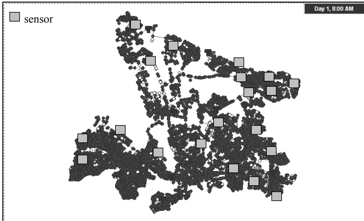
Figure 7.11 Optimal sensor locations with M = 20 for minimizing expected detection time in the case of a detection resolution of 0.3 mg/L for the Toms River WDS.
