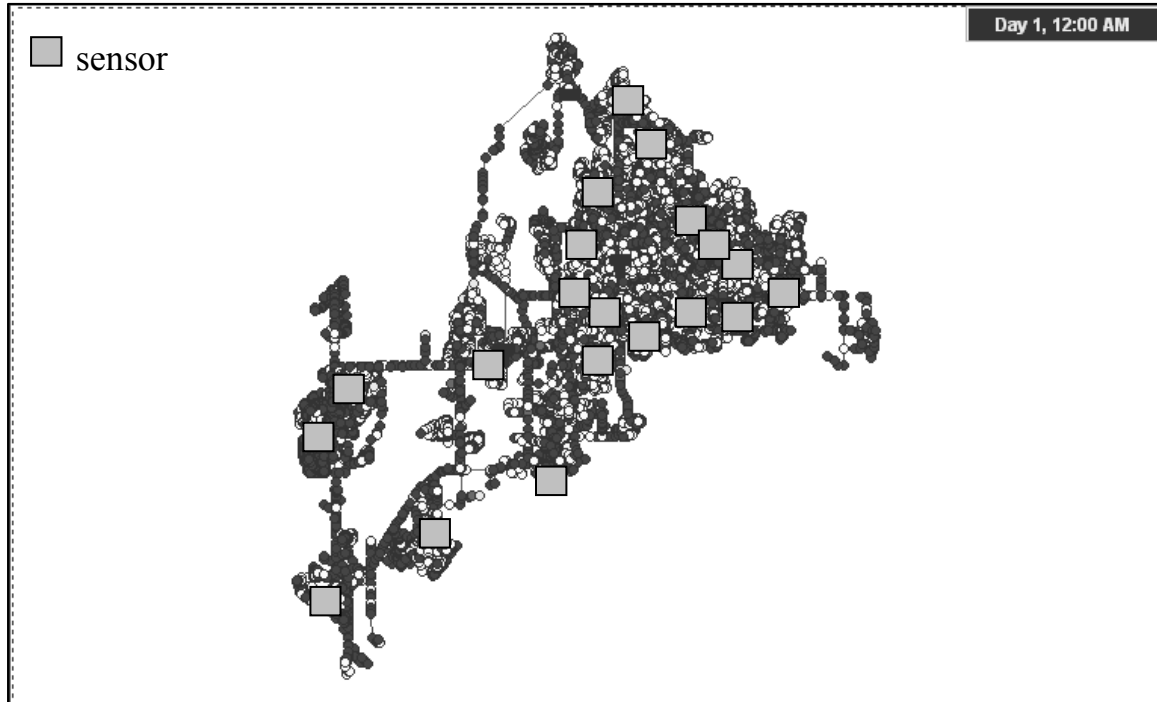
Figure 6.20 Optimal sensor locations with M = 20 for minimizing expected contaminated demand volume in the case of a 10-hour injection duration for BWSN Network 2.
