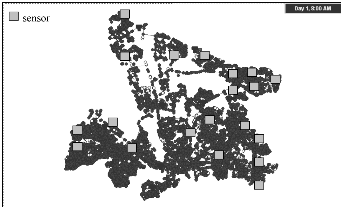
Figure 7.14 Optimal sensor locations with M = 20 for minimizing expected detection time in the case of 2 nodes injected at 2 times for the Toms River WDS.
