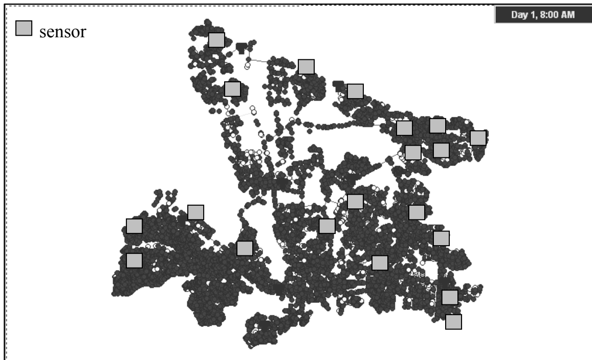
Figure 7.12 Optimal sensor locations with M = 20 for minimizing expected detection time in the case of a 10-hour injection duration for the Toms River WDS.
