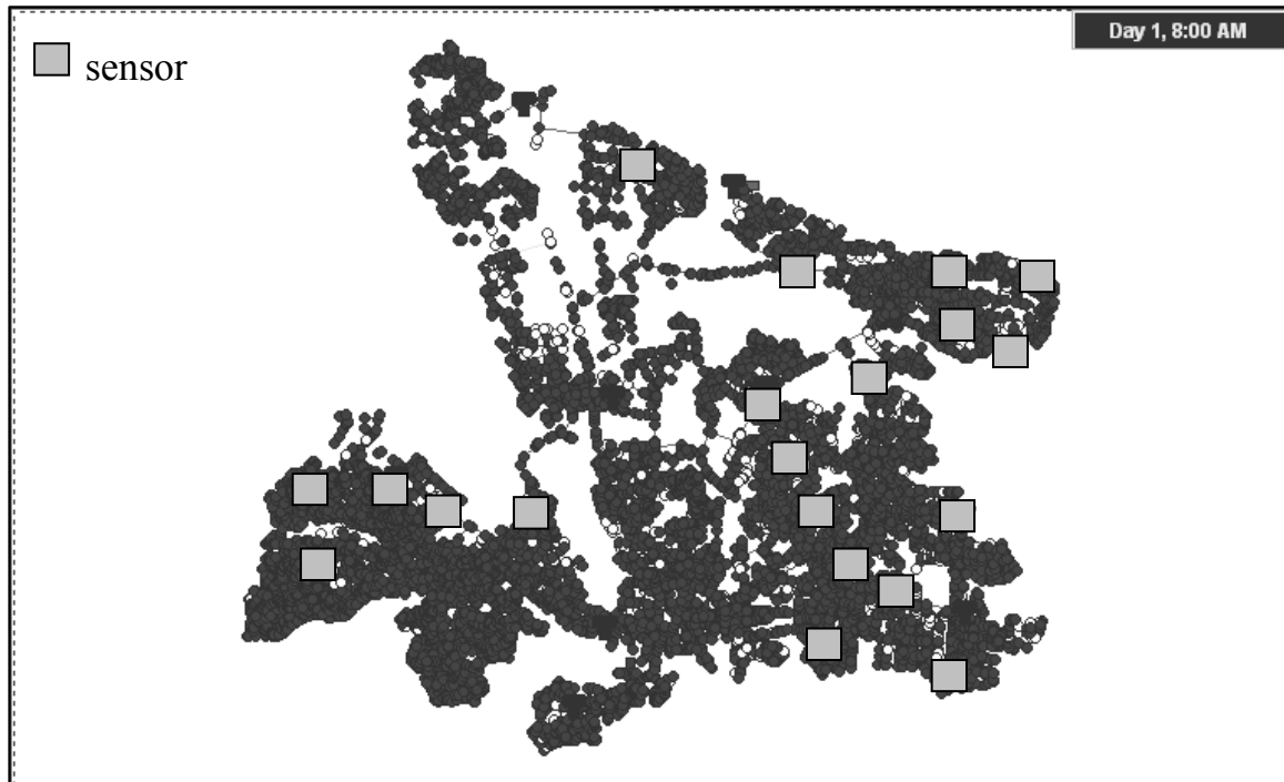
Figure 7.28 Optimal sensor locations with M = 20 for the three-prong multiobjective problem in the case of a detection resolution of 0.3 mg/L for the Toms River WDS.
