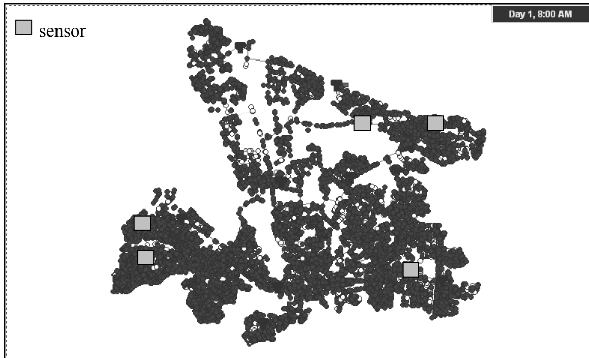
Figure 7.26 Optimal sensor locations with M = 5 for the three-prong multiobjective problem in the default attack case for the Toms River WDS.
