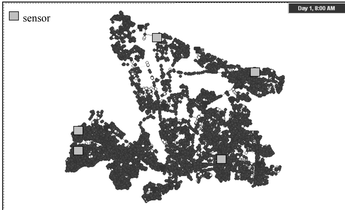
Figure 7.9 Optimal sensor locations with M = 5 for minimizing expected detection time in the default attack case for the Toms River WDS.
