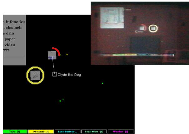
Figure 1. The browser in default *link awareness* mode (for clarity, a screen-capture from the HMD is displayed on the left, in addition to a small image taken through the HMD on the right). If any links are near the center of the display, the one closest to the center has its description displayed. The link changes to a small thumbnail (10cm in world coordinates) to provide the user with more information about its content, and a countdown begins till it is gaze-selected.
