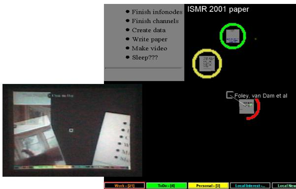
Figure 4. The small image to the left shows what the user sees when they look down and slightly to the right. The node that is currently gaze-selected (the picture) is to the left, and another node (a checklist) has been saved and is to the right. The large image is a screen shot showing what would be displayed on the HMD if the user looked straight ahead at the information nodes. The green circle indicates the saved node, the yellow circle indicates the gaze-selected node.
