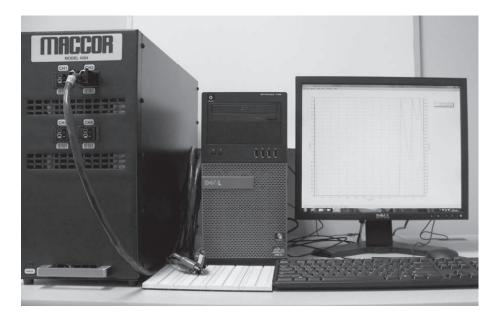
Figure 8: Maccor supercapacitor testing system.
