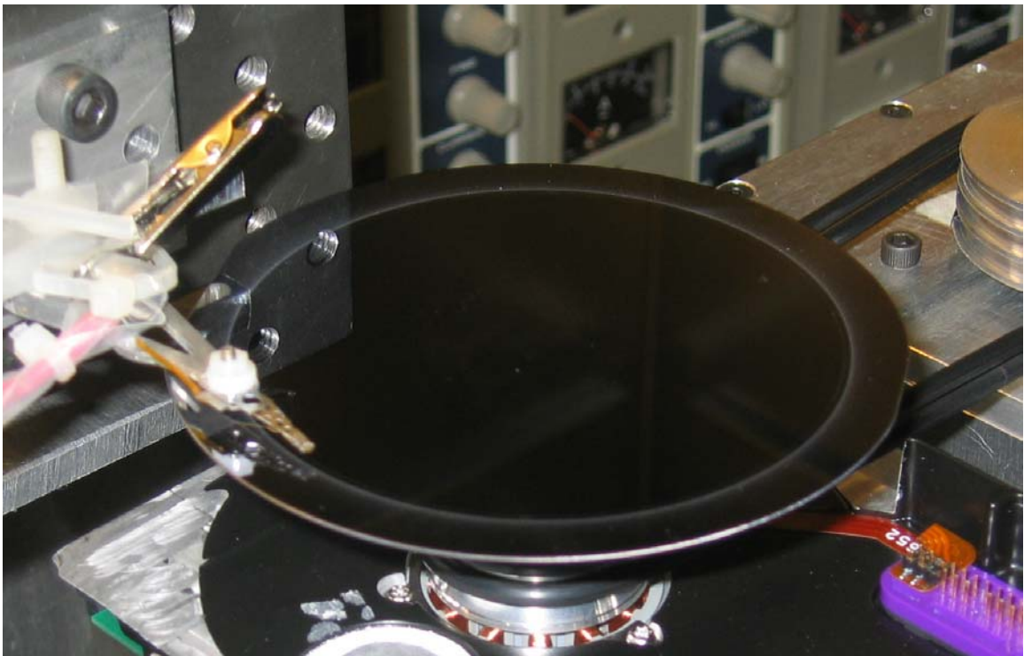
Figure 30: Example of Wear Track Formation and Si Wafer Configuration
