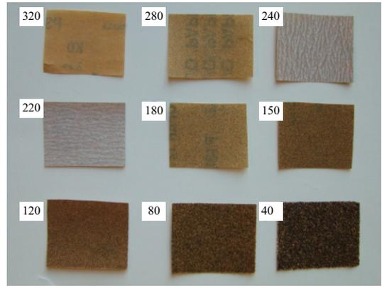
Fig. 10. Sandpapers used in texture discrimination test: Numbers indicate US CAMI grit sizes.
