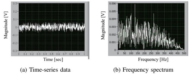
Fig. 3. Reference commands to the piezoelectric actuator: Band-limited white noise with a cutoff frequency of 300 Hz
