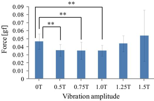
Fig. 9. Results of one-point test: Perceivable forces for 0.5T ~ 1.25T were smaller than that of the no-vibration case (0T). Statistically significant differences were observed for 0.5T ~ 1.0T (\*\* means  $p < 0.01$ ).
