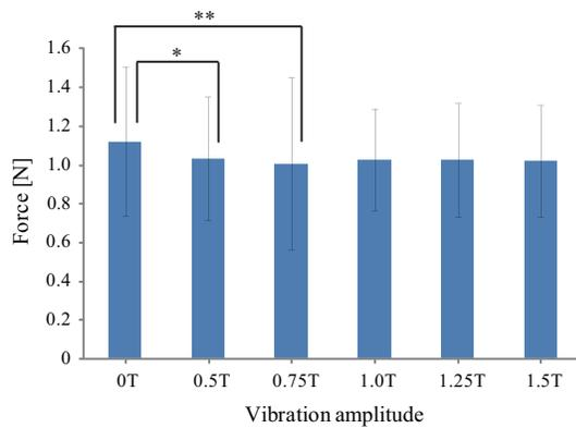
Fig. 16. Results of grasping test: Grasping forces for all of the controlled cases were smaller than that of the no-vibration case (0T). Statistically significant differences were observed for 0.5T ( $p < 0.05$ ) and 0.75T ( $p < 0.01$ ).
