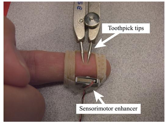
Fig. 6. Two-point discrimination test
