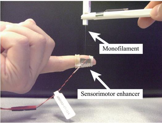
Fig. 8. One-point touch test
