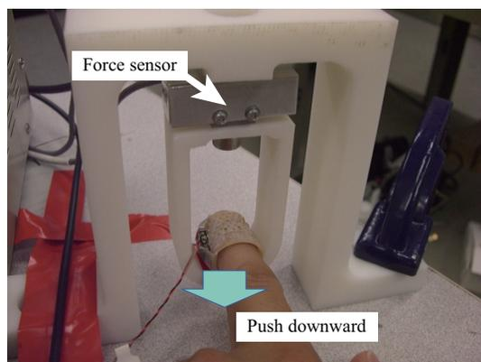
Fig. 13. Submaximal force generation test
