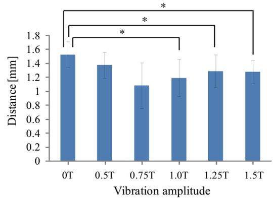
Fig. 7. Results of two-point test: Discriminable distances for conditions 0.5T ~ 1.5T were smaller than that of the no-vibration case (0T). Statistically significant differences were observed for 1.0T ~ 1.5T (\* means  $p < 0.05$ ).
