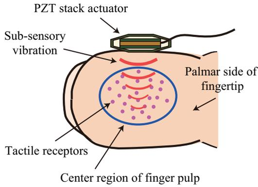
Fig. 1. Concept of the sensorimotor enhancer
