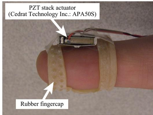
Fig. 2. Prototype sensorimotor enhancer
