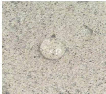
Figure 23: Hydrophobic treatment of the new material. The drop of water cannot penetrate the surface and forms a certain angle with it, characteristic of hydrophobic materials.
