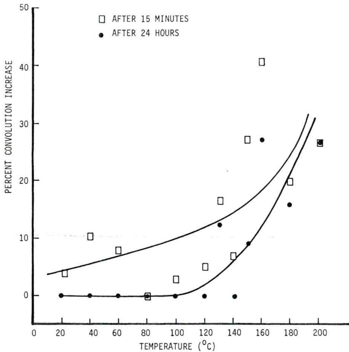
Figure 8. Convolution Change versus Temperature
