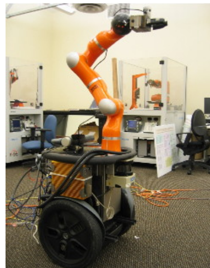
Fig. 1 The Segway RMP200 with the KUKA LWR mounted on-top. The mobile manipulation system considered here.
