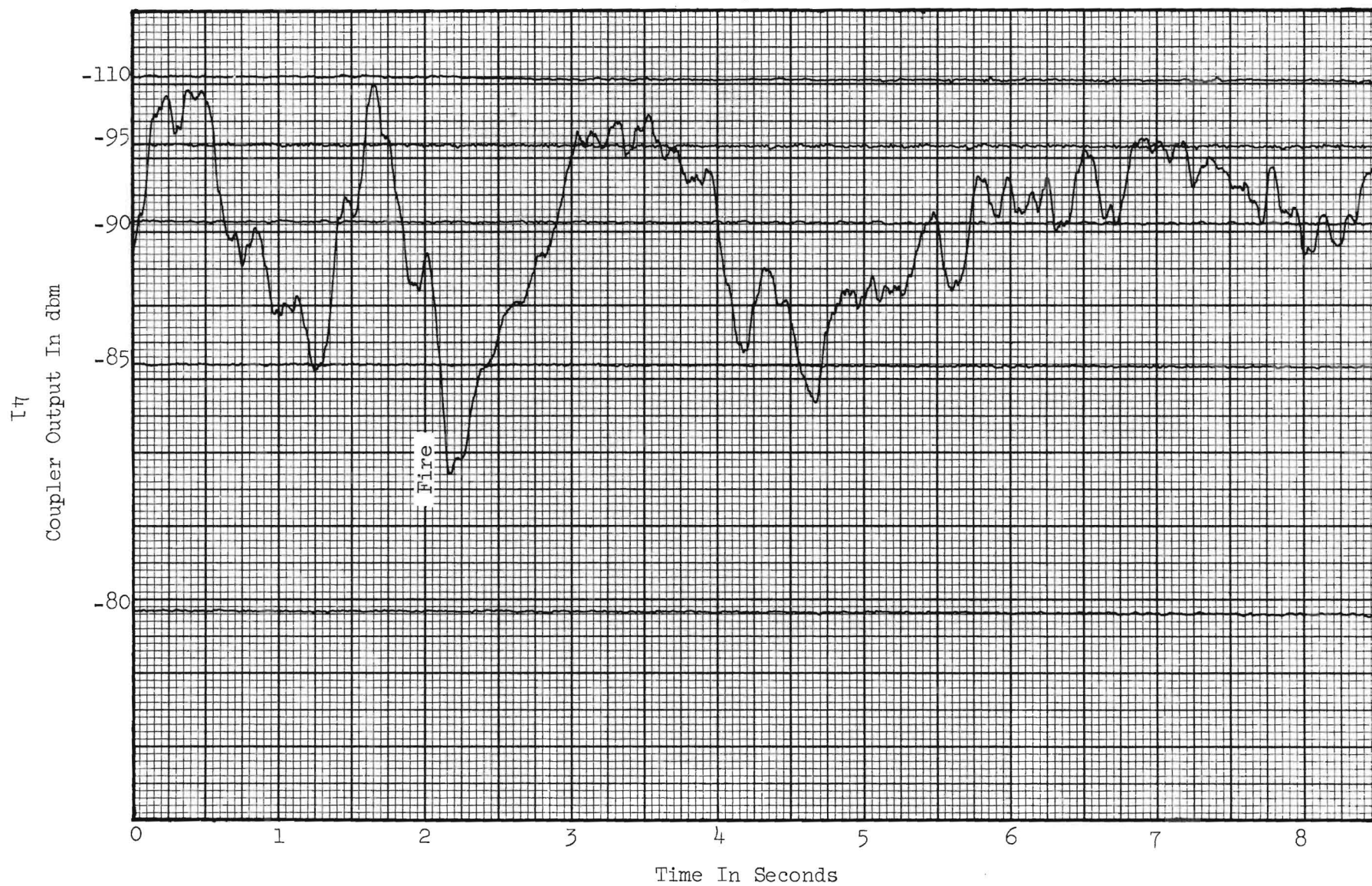
Figure 17. Recording of the 40 MHz Noise Component In the Signal Output of the Exhaust Coupler.
