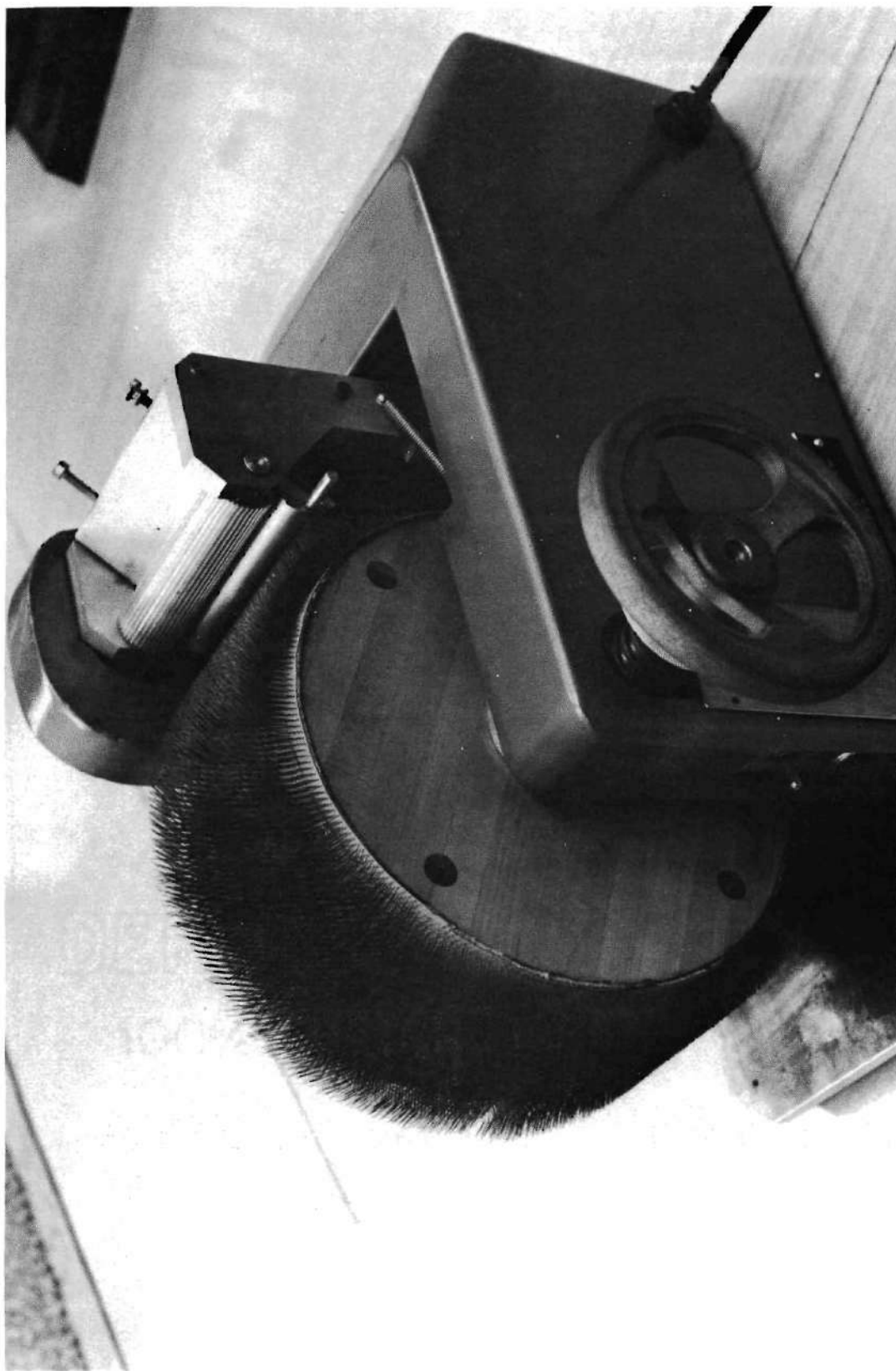
Figure 1. Custom Scientific Instruments Mechanical Cotton Sample Blender
