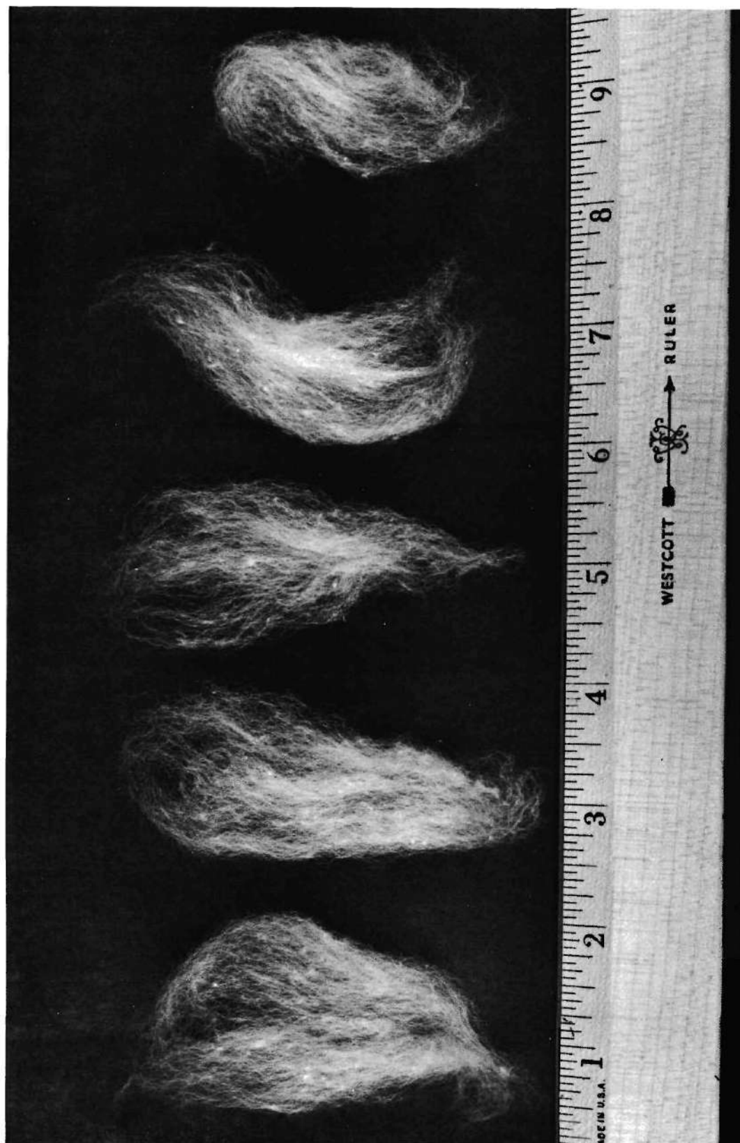
Figure 33. Average Tuft Sizes of Cotton Produced by Shirley Miniature Draw Frame
