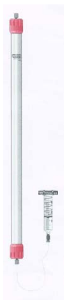
Figure B-11. Schematic illustration HPLC column with storage syringe
