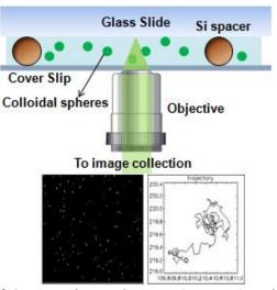
**Figure 4.1** Schematic of the experimental setup. A representative particle tracking image of the fluorescent particles obtained using microscopy is also shown.
