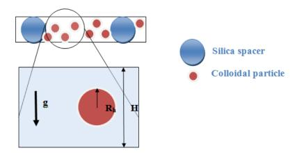
Figure 4.3 Schematic of confinement cell. *H* represents the spacer diameter, and  $R_h$  the hydrodynamic radius, respectively.
