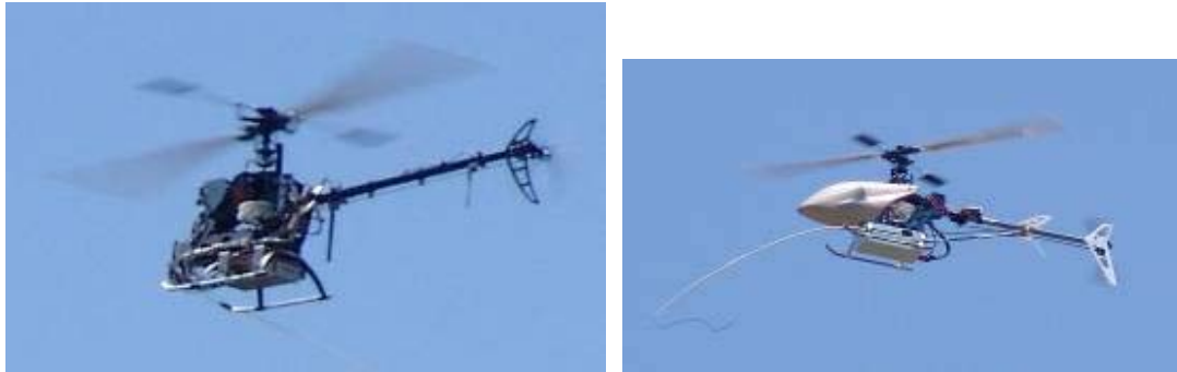
Figure 3: Two types of aircraft were utilized for testing and development under this project, (Left) a 3 kg system based on the Mikado Logo 14 hobby helicopter, (Right) a 1 kg system based on the Align T-Rex 450 hobby helicopter, the latter in cooperation with Adaptive Flight, Inc.
