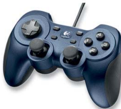
Figure 4: Typical of the operator input devices used in this work: Two two-axis joysticks on the device are used to allow the operator to adjust move the camera view up/down, left/right, and forward/backward; and to turn left/right. Letting go (centering) both sticks results in hover at the current location.
