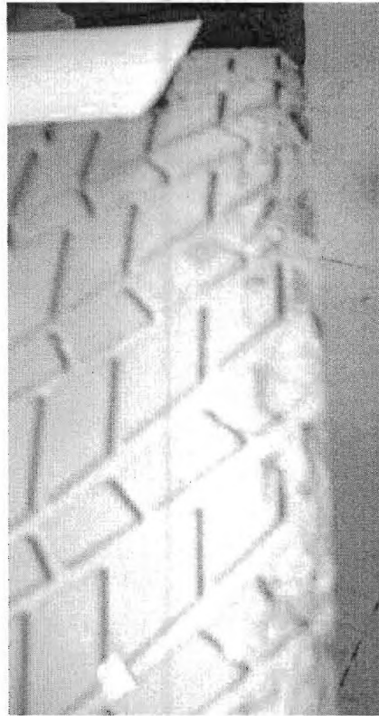
Figure 4: Extensive tread damage to a drive wheel
