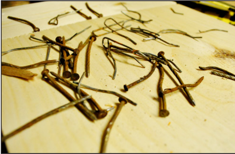
Rusty with age, these helical nails and staples should be removed from pallets.
