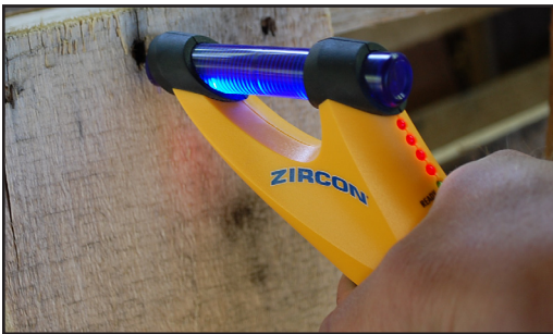
Using a hand held metal detector to locate hidden nails.
