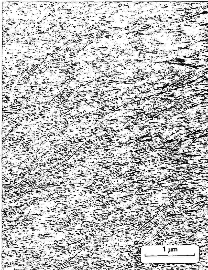
Figure 43. Balsam Fir Warty Layer Treated with Sodium Chlorite then Pectinase; Replica, TEM Plate 10124
