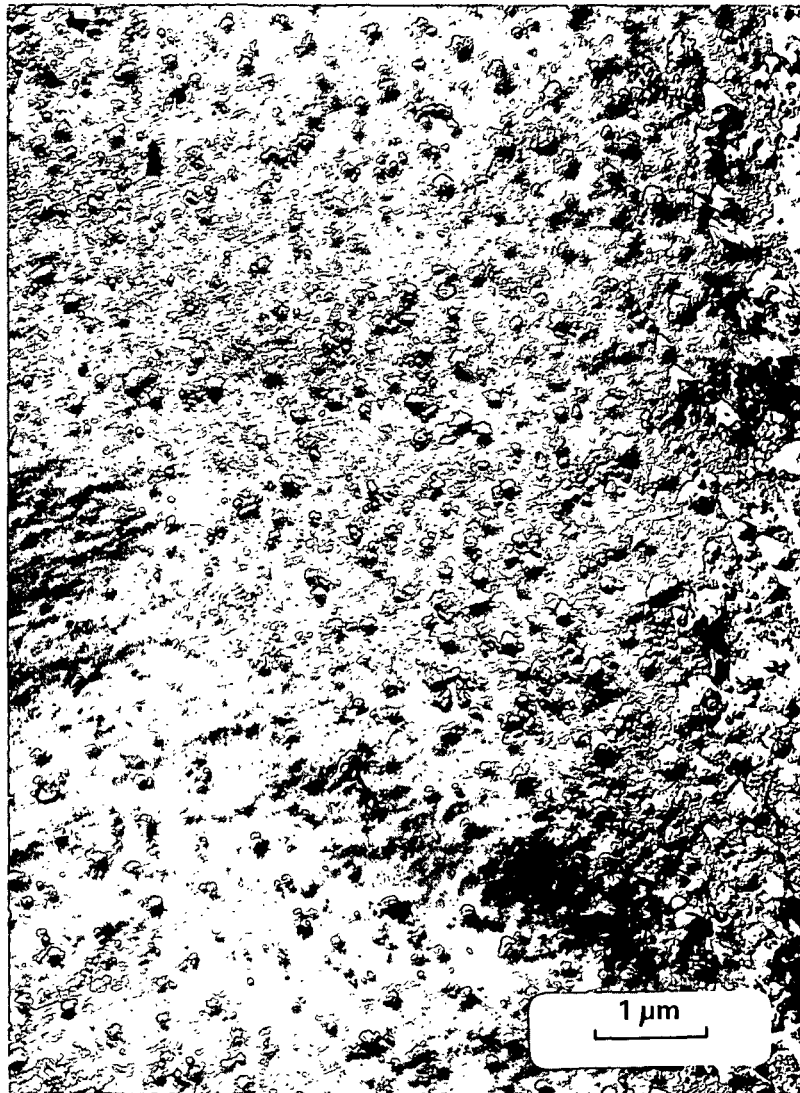
Figure 22. Radial Face and Corner Displaying Developing Warty Layer; June 12 Sample, Replica, TEM Plate 10043
