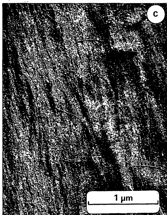
Figure 21A-21D. Inner Surface of Developing Tracheids in a Radial File Moving Inward from the Cambium: A. Primary Wall, B. S1 Layer, C. Exterior Part of S2 Layer, D. Interior Part of S2 Layer; June 12 Sample, Replica, TEM Plates 10018, 10019, 10036, and 10037
