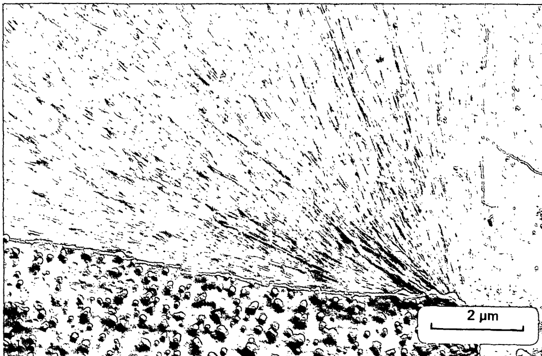
Figure 7. Warty Layer and Exposed Layers of Underlying Secondary Wall; Replica, TEM Plate 10029
