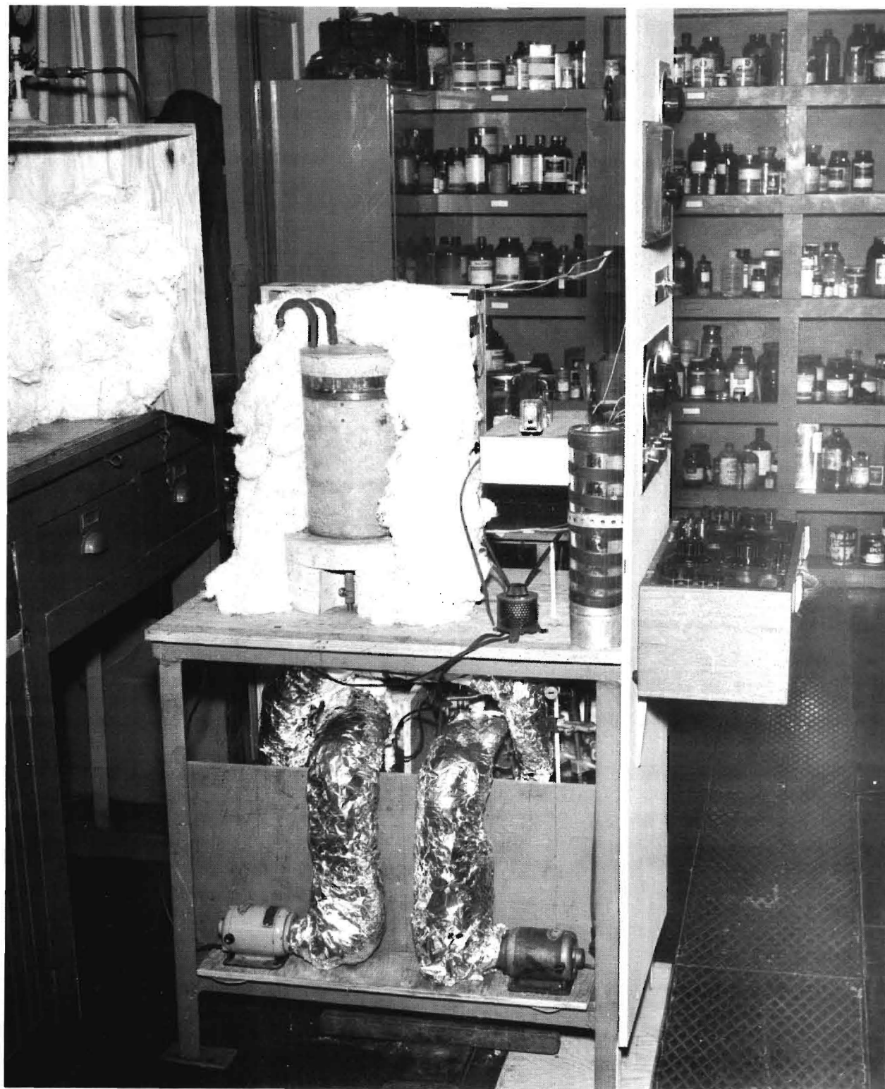
Figure 5. Side View of the Apparatus with a Portion of the Calorimeter Exposed.
